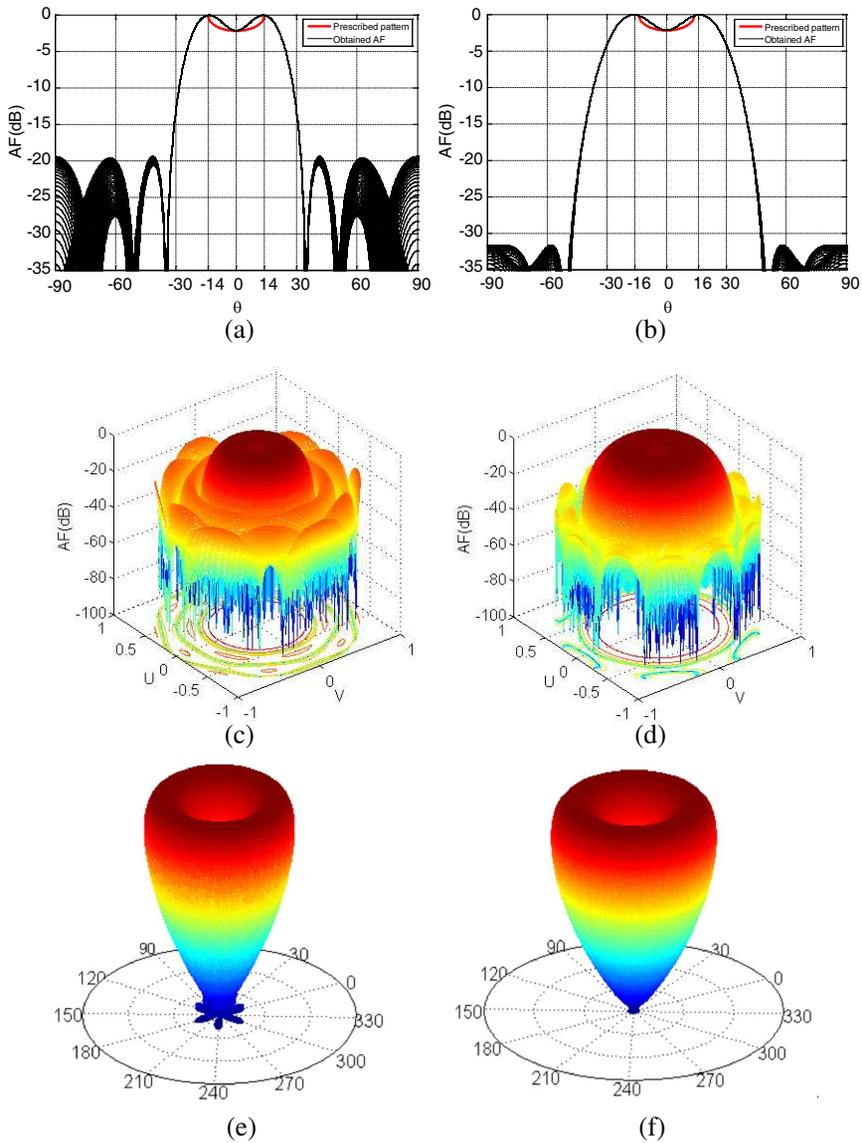
**Figure 3.** Isoflux radiation of the obtained concentric ring array. Elevation plane: (a) Case 1 and (b) Case 2. Elevation and azimuth planes in dB: (c) Case 1 and (d) Case 2. And elevation and azimuth planes in the power density of the  $AF(\theta, \varphi)$  in spherical coordinates: (e) Case 1 and (f) Case 2.
