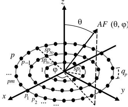
**Figure 1.** Concentric ring antenna array.
