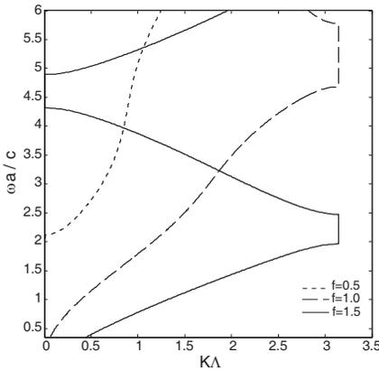
**Figure 2.** The band gap for  $a = 500 \mu\text{m}$ ,  $\theta_0 = 0$ ,  $p = 0.2$ ,  $\varepsilon_b = 4.0$  and  $\varepsilon_0 = 3.0$  for different values of  $f$ .
