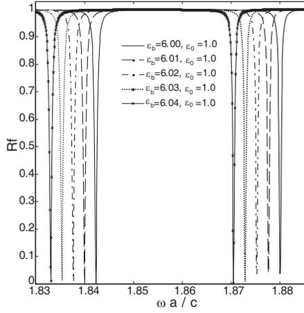
**Figure 8.** The shift of dip of reflectivity for  $a = 500 \mu\text{m}$ ,  $f = 2.0$ ,  $\theta_0 = 0$ ,  $p = 0.2$ ,  $N = 3$  and  $\varepsilon_0 = 1.0$  at different values of  $\varepsilon_b$ .
