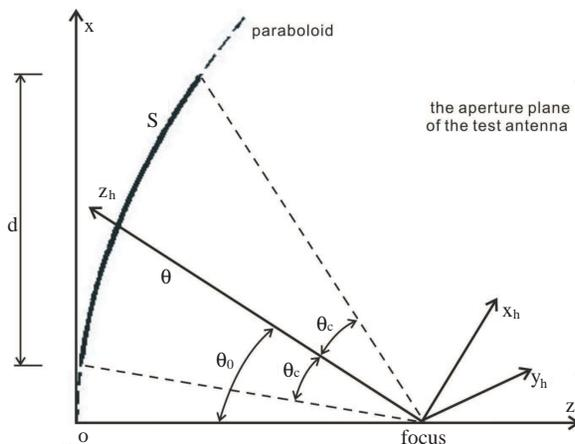
Figure 1. Offset paraboloid configuration.
