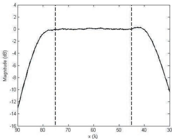
**Figure 8.** The magnitude distribution in the aperture plane of the test antenna along the axis  $x$ .
