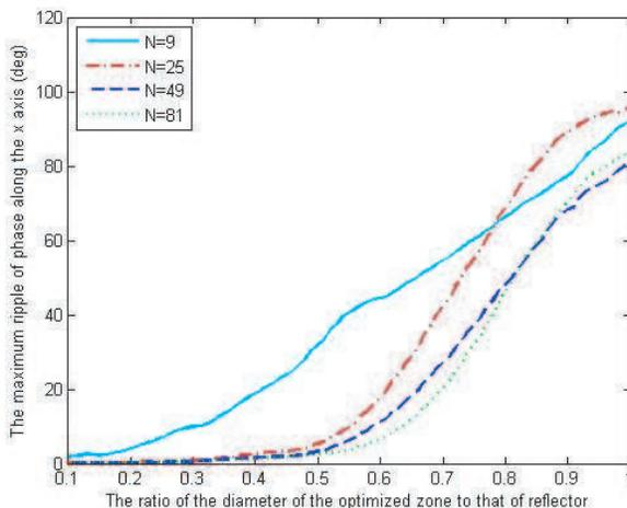
**Figure 4.** The maximum ripple of phase along the axis  $x$  for different numbers of feed scanning.
