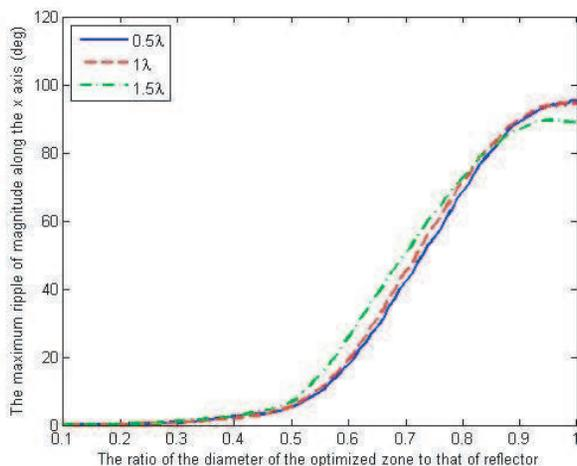
**Figure 6.** The maximum ripple of phase along the axis  $x$  for different spacings of feed scanning.
