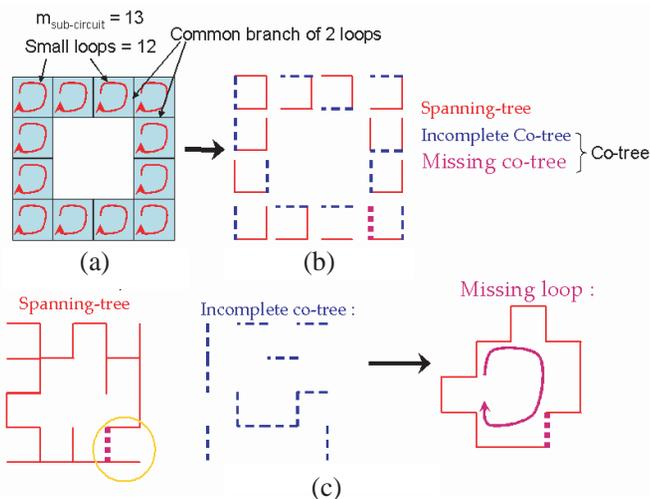
**Figure 4.** Sub-circuit loops analysis and detection of missing loops. (a) Sub-circuit created from small loops. (b) Graph of sub-circuit. (c) Search of missing loop.
