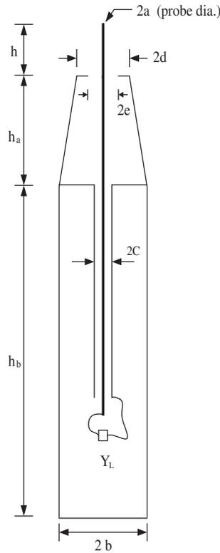
**Figure 5.** The cross sectional view of the structure (dimensions are:  $h = 5.35$  cm,  $h_b = 118.7$  cm,  $h_a = 14.6$  cm,  $a = 0.0787$  cm,  $b = 7.875$  cm,  $c = 0.2286$  cm,  $d = 4.25$  cm,  $e = 2.25$  cm.)
