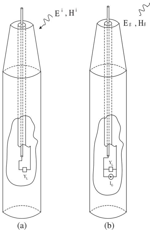
**Figure 1.** The mock-missile. (a) Excited by a plane wave, reception problem. (b) Excited through a coaxial probe, radiation problem.
