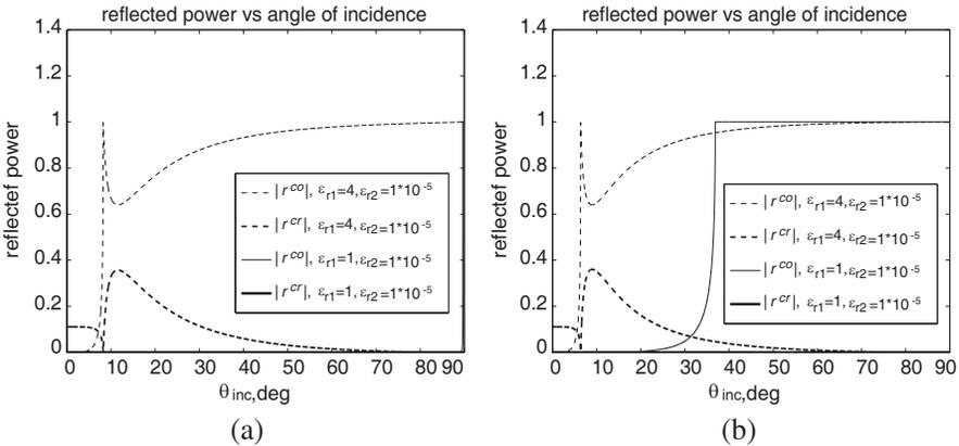
**Figure 5.** Reflected power versus angle of incidence (a) RCP incidence and (b) LCP incidence, when  $\mu_{r1} = 1, \mu_{r2} = 1 \cdot 10^{-5},$  for impedance mismatch  $\kappa_1 = \kappa_2 = 0.25,$  for impedance matching  $\kappa_1 = 0.25,$  and  $\kappa_2 = 0.75$ .
