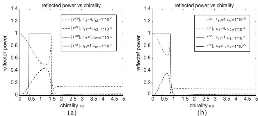
**Figure 6.** Reflected power verses chirality of the medium II (a) RCP incidence and (b) LCP incidence, when  $\kappa_1 = 0.25$ ,  $\theta_{inc} = 45^\circ$ ,  $\mu_{r1} = 1$ , and  $\mu_{r2} = 1 \cdot 10^{-5}$ .
