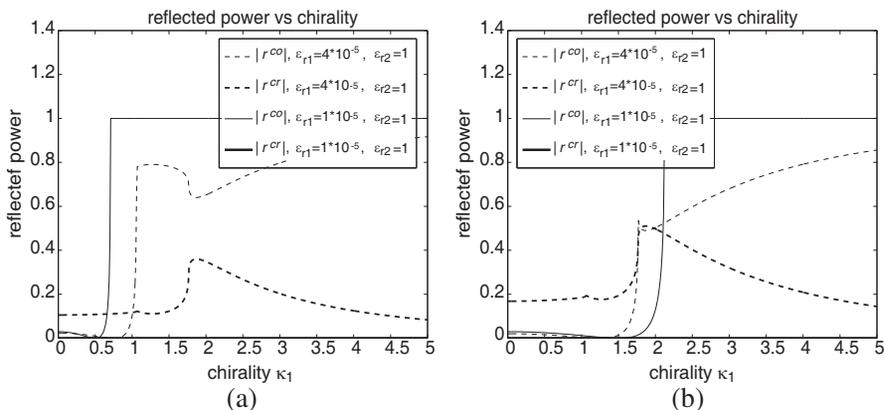
**Figure 10.** Reflected power versus chirality of medium I (a) RCP incidence and (b) LCP incidence, when  $\kappa_2 = 0.25$ ,  $\theta_{inc} = 45^\circ$ ,  $\mu_{r2} = 1$ , and  $\mu_{r1} = 1 * 10^{-5}$ .
