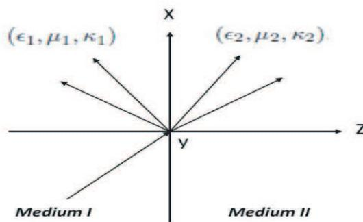
**Figure 1.** Reflection and transmission in chiral media: Incident RCP/LCP, Reflected LCP and RCP, Refracted LCP and RCP.
