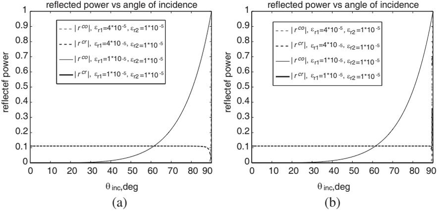
**Figure 11.** Reflected power versus angle of incidence (a) RCP incidence and (b) LCP incidence, when  $\mu_{r1} = 1 \times 10^{-5}$ ,  $\mu_{r2} = 1 \times 10^{-5}$ , for impedance mismatch  $\kappa_1 = 0.25$ ,  $\kappa_2 = 0.25$ , for impedance matching  $\kappa_1 = 0.25$ , and  $\kappa_2 = 0.75$ .
