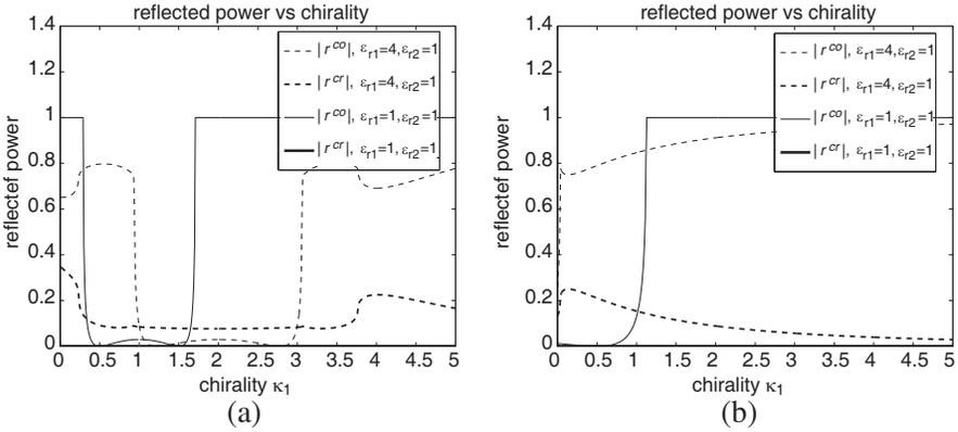
**Figure 4.** Reflected power versus chirality of the medium I (a) RCP incidence and (b) LCP incidence, when  $\kappa_2 = 0.25, \mu_{r1} = \mu_{r2} = 1,$  and  $\theta_{inc} = 45^\circ$ .
