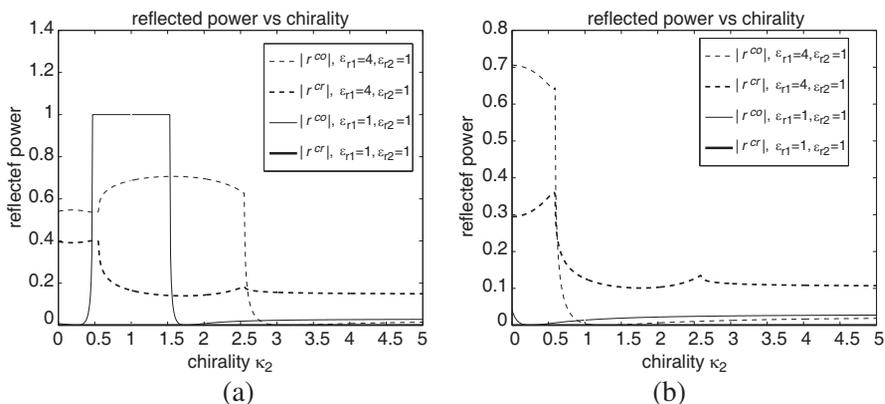
**Figure 3.** Reflected power verses chirality of the medium II (a) RCP incidence and (b) LCP incidence, when  $\kappa_1 = 0.25, \mu_{r1} = \mu_{r2} = 1$ , and  $\theta_{inc} = 45^\circ$ .
