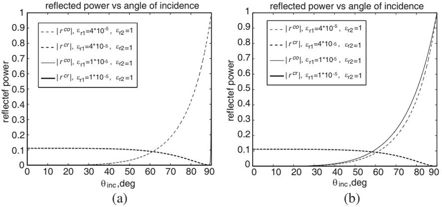
**Figure 8.** Reflected power versus angle of incidence (a) RCP incidence and (b) LCP incidence, when  $\mu_{r2} = 1$ ,  $\mu_{r1} = 1 * 10^{-5}$ , for impedance mismatch  $\kappa_1 = \kappa_2 = 0.25$ , for impedance matching  $\kappa_1 = 0.25$ , and  $\kappa_2 = 0.75$ .
