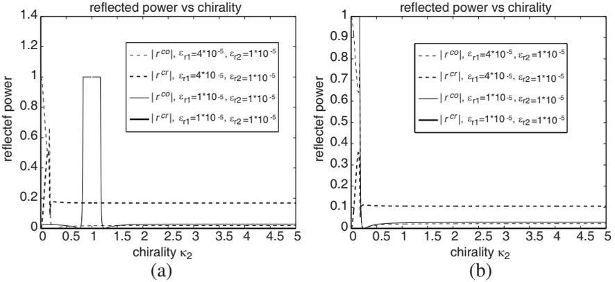
**Figure 12.** Reflected power versus chirality of the medium II (a) RCP incidence and (b) LCP incidence, when  $\kappa_1 = 0.25$ ,  $\mu_{r1} = 1 \times 10^{-5}$ ,  $\mu_{r2} = 1 \times 10^{-5}$ , and  $\theta_{inc} = 45^\circ$ .
