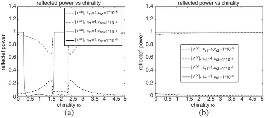
**Figure 7.** Reflected power versus chirality of medium I (a) RCP incidence and (b) LCP incidence, when  $\kappa_2 = 0.25$ ,  $\theta_{\text{inc}} = 45^\circ$ ,  $\mu_{r1} = 1$ , and  $\mu_{r2} = 1 * 10^{-5}$ .
