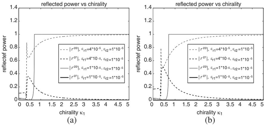
**Figure 13.** Reflected power versus chirality of the medium I (a) RCP incidence and (b) LCP incidence, when  $\kappa_2 = 0.25$ ,  $\mu_{r1} = 1 * 10^{-5}$ ,  $\mu_{r2} = 1 * 10^{-5}$ , and  $\theta_{inc} = 45^\circ$ .
