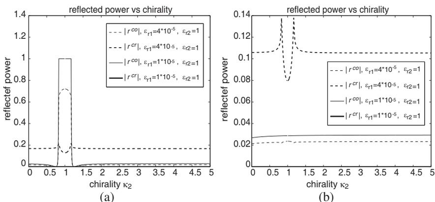
**Figure 9.** Reflected power versus chirality of the medium II (a) RCP incidence and (b) LCP incidence, when  $\kappa_1 = 0.25$ ,  $\theta_{inc} = 45^\circ$ ,  $\mu_{r2} = 1$ , and  $\mu_{r1} = 1 * 10^{-5}$ .
