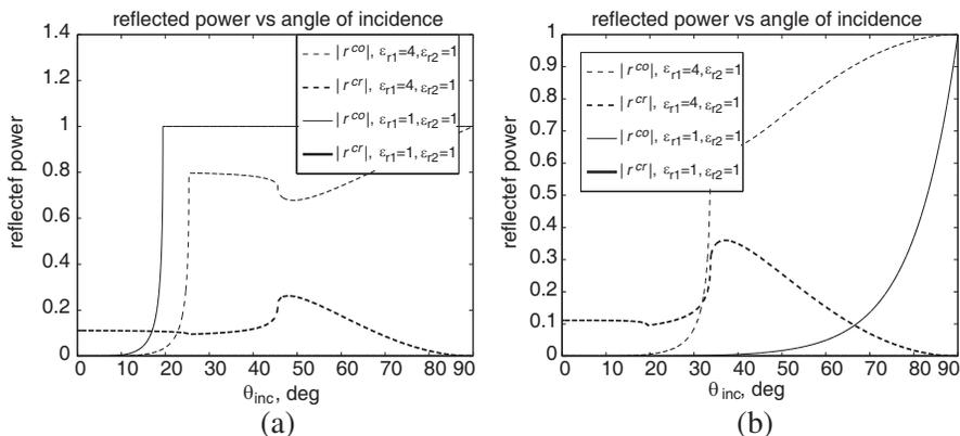
**Figure 2.** Reflected power verses angle of incidence (a) RCP incidence and (b) LCP incidence, when  $\mu_{r1} = \mu_{r2} = 1$ , for impedance mismatch  $\kappa_1 = \kappa_2 = 0.25$  and for impedance matching  $\kappa_1 = 0.25, \kappa_2 = 0.75$ .
