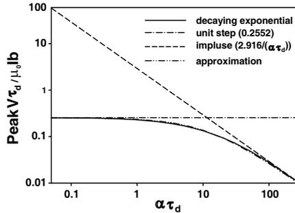
**Figure 4.** Peak voltage bound for direct strikes.
