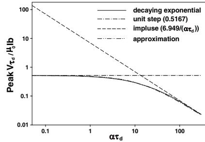
**Figure 8.** Peak voltage bounds for direct strikes ( $\mu = 10\mu_0$ ).
