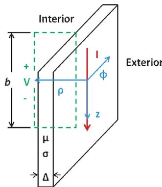
**Figure 2.** Direct lightning strike to an insulated cable parallel to the enclosure wall and a maximum coupling loop.
