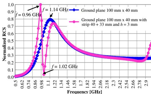
**Figure 6.** Comparison of the normalized RCS for a ground plane of 100 mm × 40 mm and the same ground plane with the metallic strip as shown in Fig. 5.
