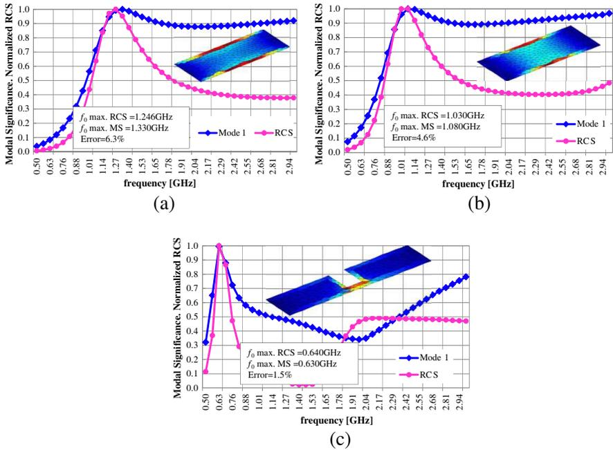
**Figure 2.** Comparison between normalized RCS and modal significance (MS); (a) bar-type platform 100 mm × 40 mm; (b) smartphone platform 120 mm × 50 mm; (c) clamshell 80 mm × 40 mm for each upper and lower board.
