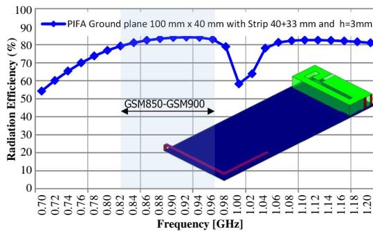
**Figure 8.** Simulated radiation efficiency for a PIFA on a ground plane 100 mm  $\times$  40 mm and a metallic strip 40 mm + 33 mm and 3 mm height.
