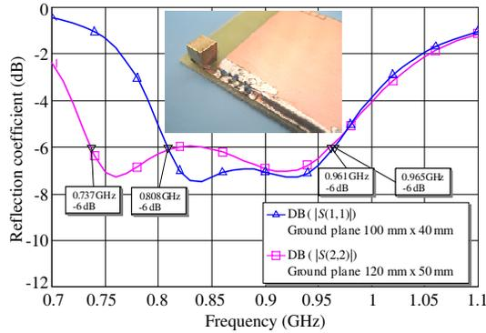
**Figure 3.** Measured reflection coefficient for a non-resonant element of  $5 \text{ mm} \times 5 \text{ mm} \times 5 \text{ mm}$  regarding two different platforms.
