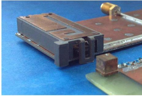
**Figure 4.** Comparison of a PIFA and a ground plane booster both for GSM850-GSM900 operation. Size for the PIFA is  $40 \text{ mm} \times 15 \text{ mm} \times 6 \text{ mm}$  whereas the ground plane booster is only  $5 \text{ mm} \times 5 \text{ mm} \times 5 \text{ mm}$ .
