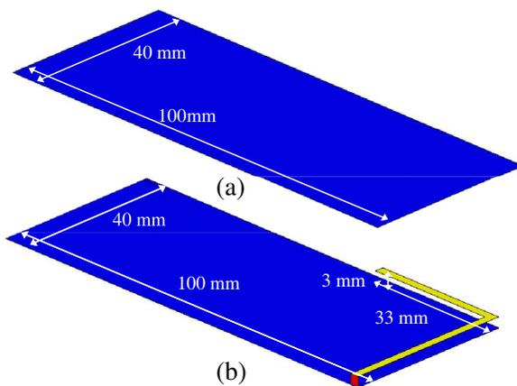
**Figure 5.** (a) A ground plane of 100 mm × 40 mm and (b) the same ground plane having a metallic strip of 40 mm + 33 mm and 3 mm height. Both ground planes are supported by a thin dielectric slab of 1 mm thick with  $\epsilon_r = 4.15$ .
