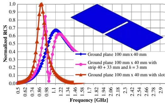
**Figure 9.** Comparison of RCS for three different ground planes: 100 mm × 40 mm, 100 mm × 40 mm with a metallic strip as shown in Fig. 5, and a ground plane 100 mm × 40 mm with slot 38 mm long and 3 mm width. The plane wave impinges the ground plane as shown in Fig. 1. All ground planes are etched on a thin dielectric slab of 1 mm thick and  $\epsilon_r = 4.15$ .
