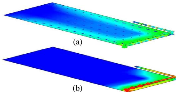
**Figure 7.** Induced current (A/m) for a plane wave excitation as in Fig. 1 at (a)  $f = 0.96$  GHz and (b)  $f = 1.02$  GHz. Same maximum and dynamic range is used for both plots.
