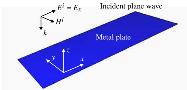
**Figure 1.** The metal plate is representative of a ground plane associated to a bar-type wireless handheld device.
