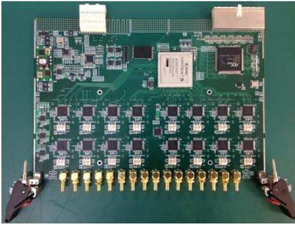
**Figure 4.** The data acquisition unit in BHU-2D.
