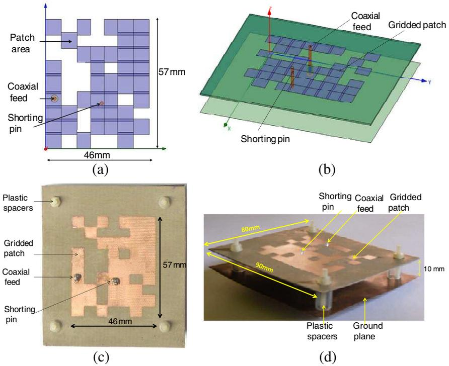
**Figure 6.** The optimized (hexa band) MPA with a shorting pin and a 10 mm air gap. (a) Top view. (b) 3D view. (c) Photo of the fabricated antenna (top view). (d) Photo of the fabricated antenna (3D view).
