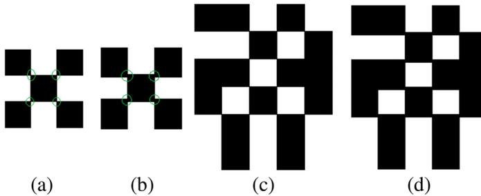
**Figure 2.** (a) Traditional on/off building block with infinitesimal connections. (b) Proposed scheme with overlapping obtained by shifting the cells along the vertical axis. (c) An example of a possible structure obtained with GA using infinitesimal connections. (d) A possible structure with overlapping as proposed.
