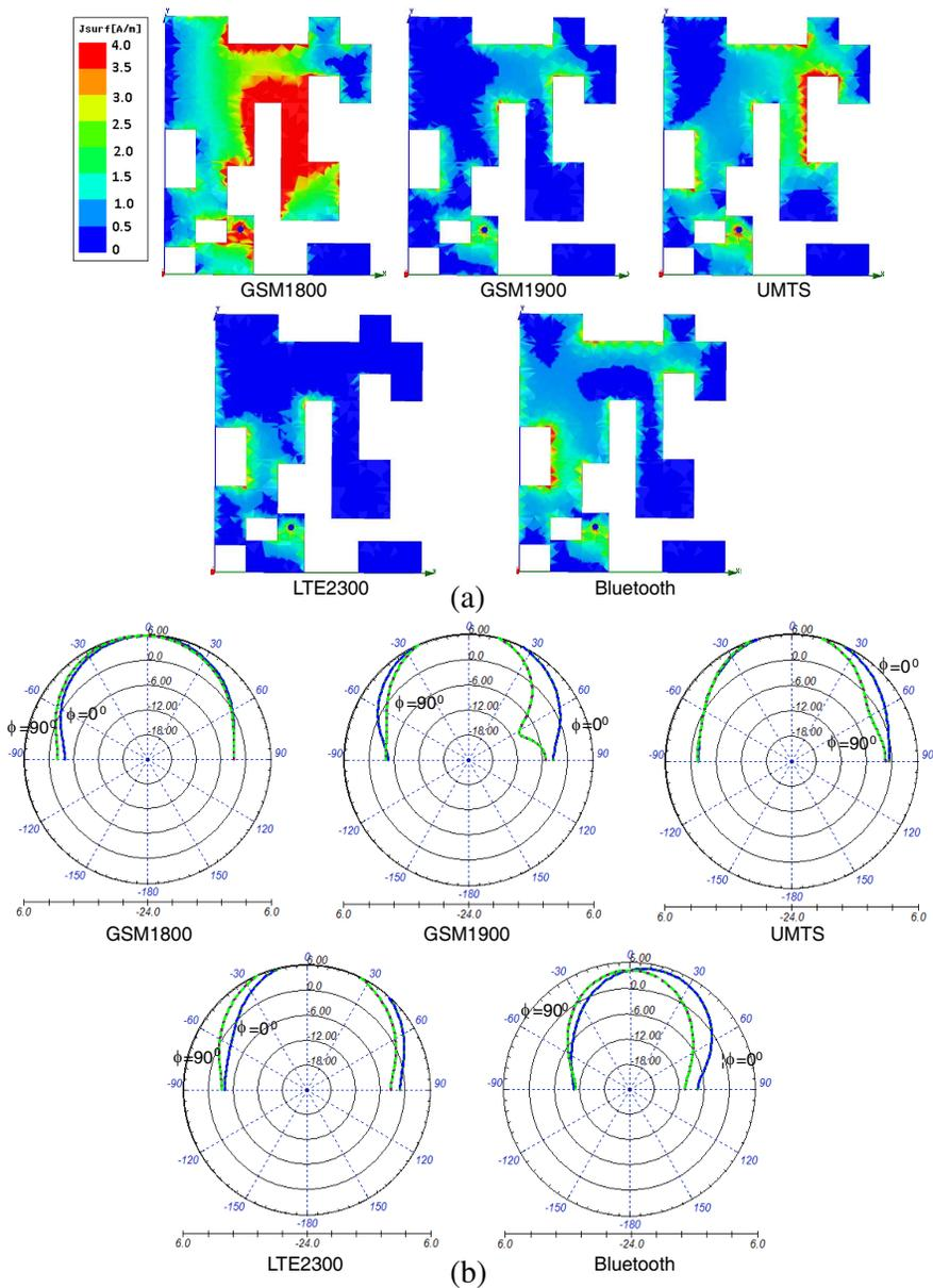
**Figure 5.** Simulation results of the penta band MPA (air gap with 10 mm). (a) Current distribution at center frequency of each band. (b) Radiation patterns for  $\phi = 0^\circ$  and  $\phi = 90^\circ$  planes at center frequency of each band.
