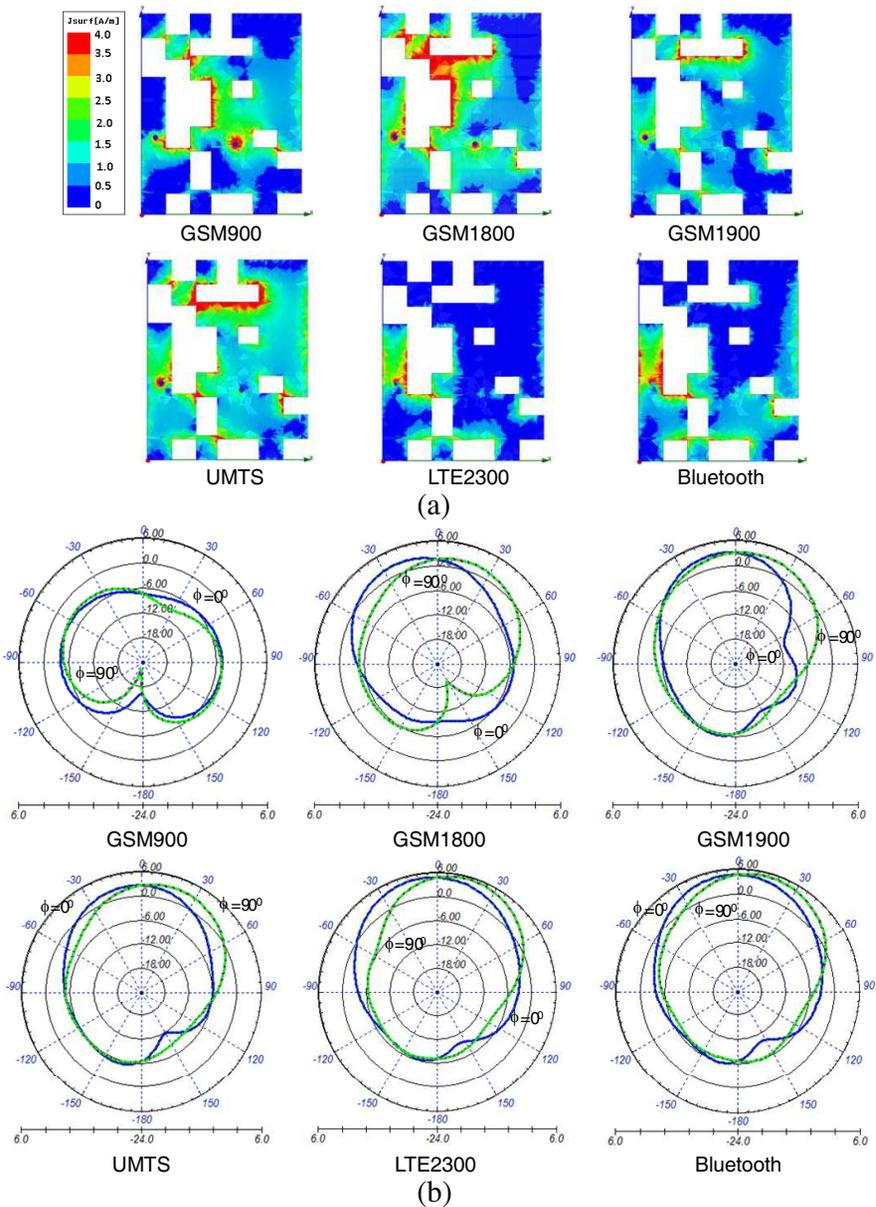
**Figure 8.** Simulation results of the hexa band MPA (a) current distribution at center frequency of each band. (b) Radiation patterns for  $\phi = 0^\circ$  and  $\phi = 90^\circ$  planes at center frequency of each band.
