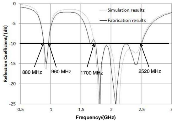
**Figure 7.** Reflection coefficient of the hexa band MPA.
