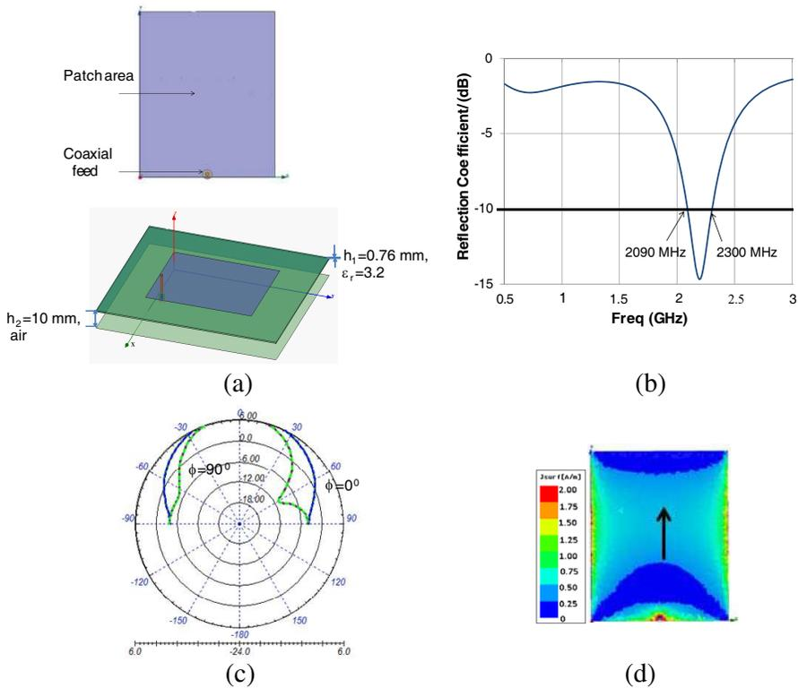
**Figure 3.** Simulation results of the rectangular shaped patch. (a) Top view and 3-D view of the MPA. (b) Reflection coefficient. (c) Radiation pattern. (d) Current distribution (the black arrow indicates the direction of current).
