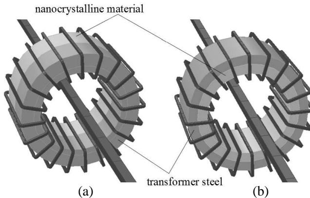
**Figure 1.** The 3D models of the measuring current transformers 100 A/5 A, (a) materials joined axially (one-by-one), and (b) radially (one inside the second) 1-transformer steel 2-nanocrystalline material.
