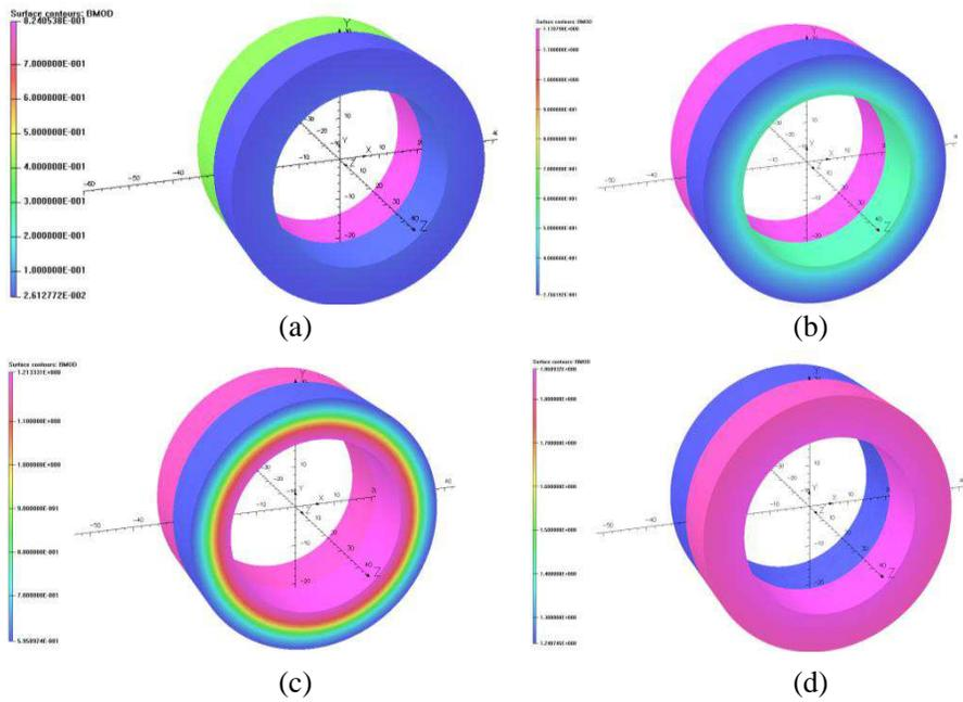
**Figure 9.** Magnetic flux density distributions [T] of measuring current transformers version C with core joined axially two materials (steel and nanocrystalline) at the primary current equal, (a) 0.2 A, (b) 1 A, (c) 1.5 A, (d) 200 A.
