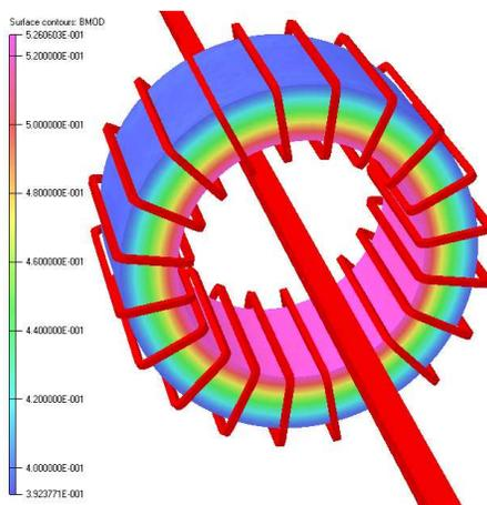
**Figure 3.** Magnetic flux density distributions [T] of measuring current transformers with core made from nanocrystalline material at the rated primary current  $I_{pn} = 100$  A and burden  $S_n = 2.5$  VA ( $\cos \varphi = 0.8$ ).
