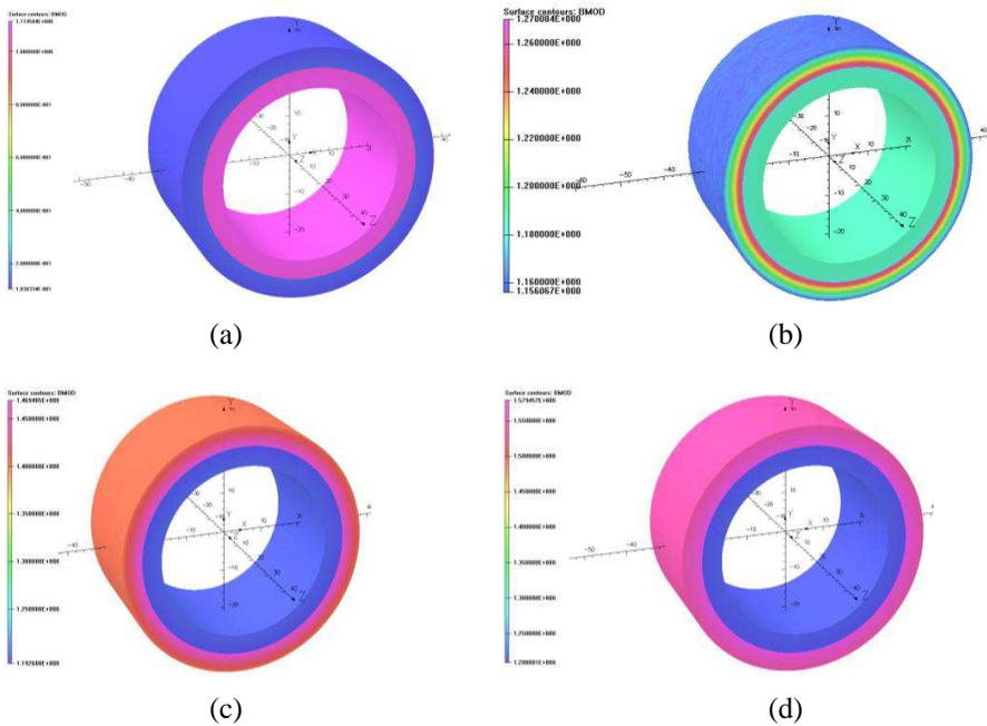
**Figure 8.** Magnetic flux density distributions [T] of measuring current transformers version C with core joined radially two materials (steel and nanocrystalline) at the primary current equal, (a) 0.5 A, (b) 2 A, (c) 30 A, (d) 200 A.
