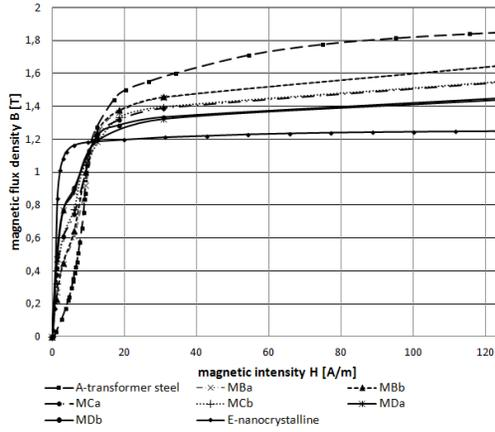
**Figure 10.** Equivalent magnetic characteristics of cores consisting of different proportions of two different connected magnetic materials (A, B, C, D, E) (total dimensions of core are constant) computed using the field-and-circuit method, (a) materials joined axially, and (b) radially.
