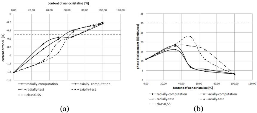
**Figure 11.** Comparison of the current errors and phase displacements for the current transformers with a core combined axially and radially vs. proportions of nanocrystalline in a joint, at the same load  $S_n = 2.5 \text{ VA}$ ,  $\cos \varphi = 0.8$  ( $I_{pn} = 100 \text{ A}$ ).
