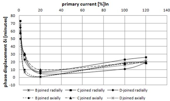
**Figure 7.** Comparison current error and phase displacement characteristics for the current transformers with a core combined axially and radially and different joint proportions (B, C, D), at the same load  $S_n = 2.5 \text{ VA}$ ,  $\cos \varphi = 0.8$  ( $I_{pn} = 100 \text{ A}$ )).
