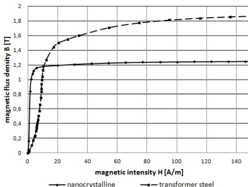
**Figure 2.** Magnetic characteristics of used core materials (test).
