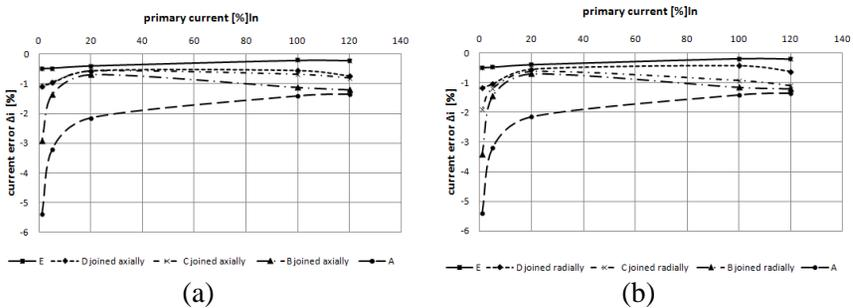
**Figure 6.** Results from tests of current error for the current transformers with combined core using different proportions of steel and nanocrystalline material, at the same load  $S_n = 2.5 \text{ VA}$ ,  $\cos \varphi = 0.8$  ( $I_{pn} = 100 \text{ A}$ ), (a) materials joined axially, and (b) radially.
