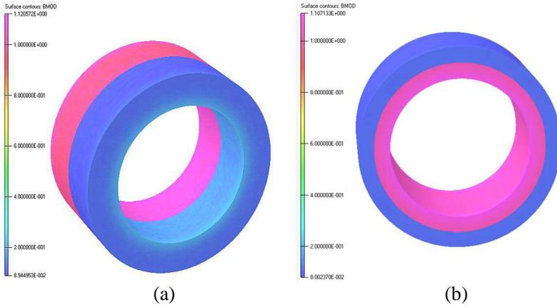
**Figure 5.** Magnetic flux density distributions [T] of measuring current transformers version C with the core made from combined steel and nanocrystalline material at the same primary current, (a) materials joined axially, and (b) radially.
