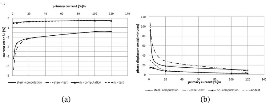
**Figure 4.** Results from computations and tests for the current transformers with the core made from transformer steel and nanocrystalline material at the same load  $S_n = 2.5$  VA,  $\cos \varphi = 0.8$  ( $I_{pn} = 100$  A), (a) current error, and (b) phase displacement characteristics of the current transformer.
