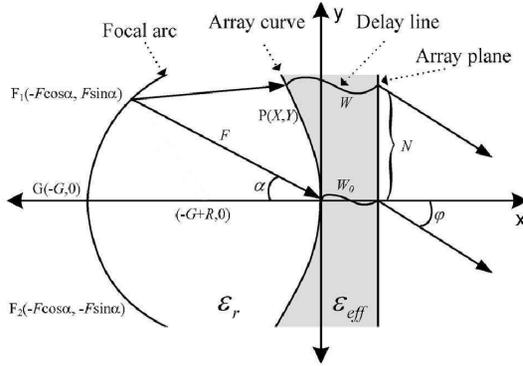
**Figure 1.** Microwave Rotman Lens geometry and design parameters [13].
