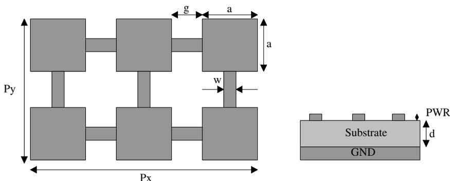
**Figure 1.** Top and side view of a  $3 \times 2$  planar EBG structure.
