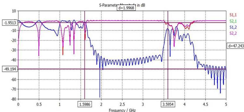
Figure 5.  $|S_{21}|$  of a power plane with & without EBG structure.
