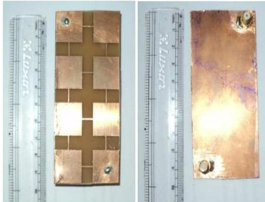
**Figure 4.** Top and Bottom view of the prototype model ( $2 \times 4$  planar EBG structure).
