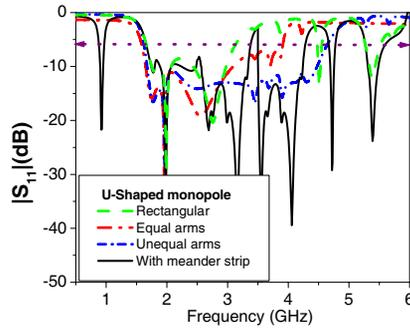
**Figure 2.** Simulated reflection coefficient of the design procedure.
