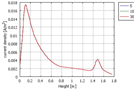
**Figure 12.** Induced current density inside the body.
