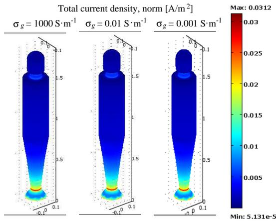
Figure 11. Induced current density on the surface of the human body for different soil conductivities ( $\epsilon_{rg} = 10$ ).
