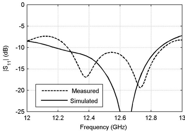
**Figure 6.** Measured and simulated reflection coefficients.
