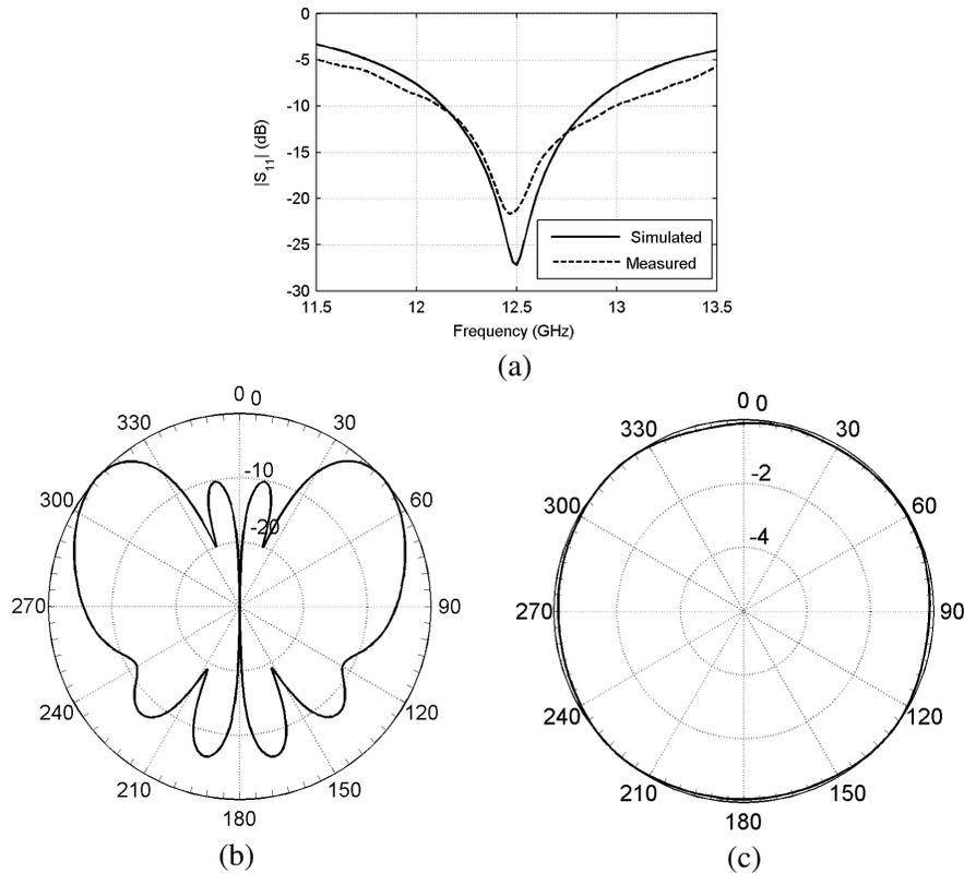
Figure 4. Reflection coefficients and radiation patterns of the conical beam element. (a) Simulated and measured results of  $|S_{11}|$ , (b) simulated normalized radiation patterns in the  $x$ - $z$  plane and (c) in the  $x$ - $y$  plane.
