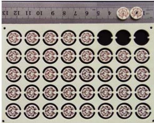
**Figure 7.** Prototypes of the fragmented versatile round tags, among which two are connected to IMPINJ Monza-4 chip (right) and ALIEN Higgs-3 chip (left).
