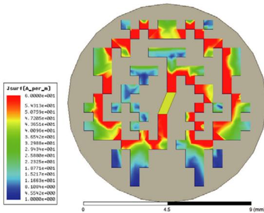
Figure 14. Current distribution on prototype of fragmented tag.
