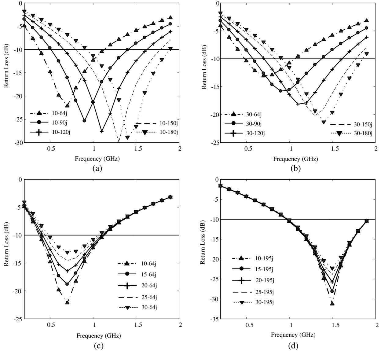
**Figure 13.** Effects of chip impedance on reflection coefficients.
