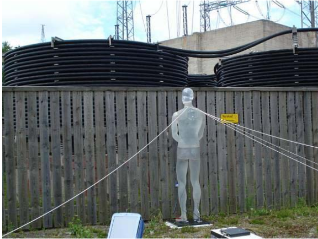
Figure 2. Human-shaped phantom in measurement place A.
