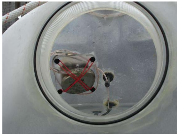
Figure 4. An example of the ICD inside the phantom (in Table 1, ICD: code 2).
