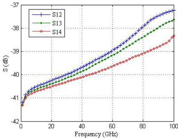
Figure 13. Coupling *S* parameters in different TSV pairs.
