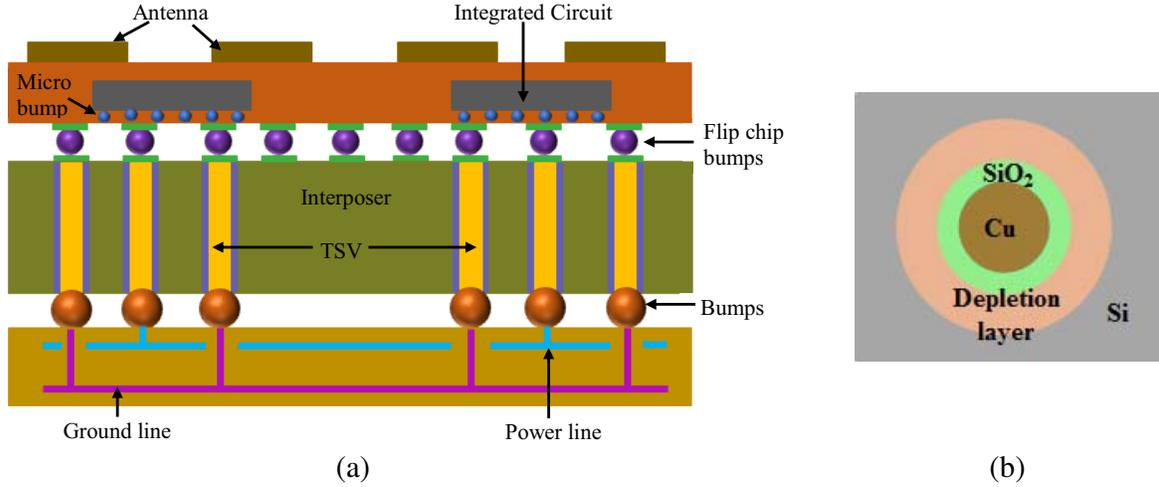
**Figure 1.** (a) 3D structure of an mmW transceiver module, and (b) cross sectional view of TSV.
