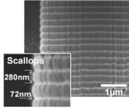
**Figure 3.** SEM image of TSV with sidewall roughness using Bosch etching [14].
