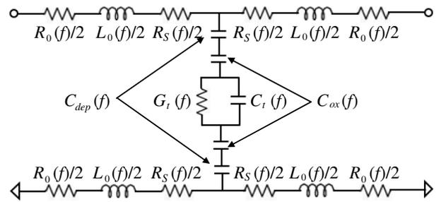
**Figure 5.** Equivalent circuit model of TSV.
