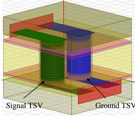
**Figure 2.** TSV pair with sidewall roughness.
