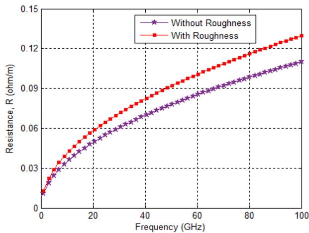
**Figure 6.** Comparison of TSV pair resistances with and without surface roughness.
