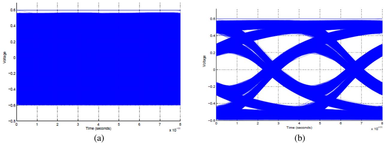
**Figure 9.** (a) Eye diagram of interposer TSV, (b) eye diagram of interposer TSV with optimized depletion capacitance.
