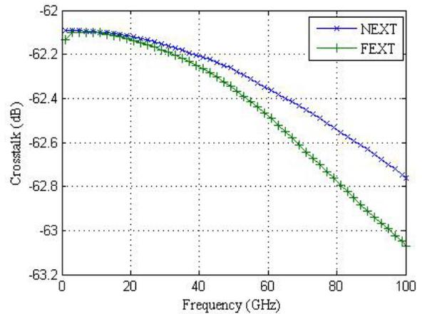
Figure 14. Signal-ground near and far end crosstalk of between two TSV pairs.
