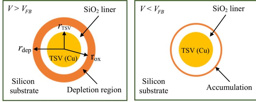
**Figure 8.** Accumulation and depletion of TSV MIS.
