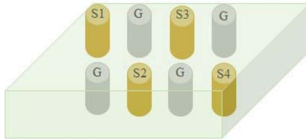
Figure 10. Different TSV configurations for coupling analysis.
