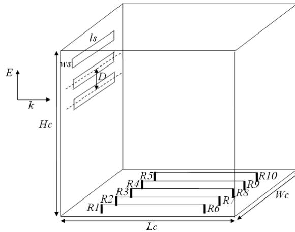
**Figure 7.** Multi-conductor lines in a shielded cavity excited by an incident wave.
