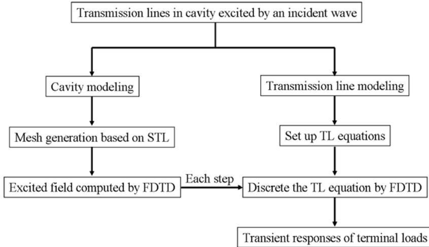
**Figure 1.** Implementation procedure of the hybrid FDTD-TL method.
