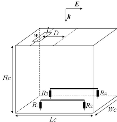
Figure 3. Two transmission lines in a shielded cavity excited by an incident wave.
