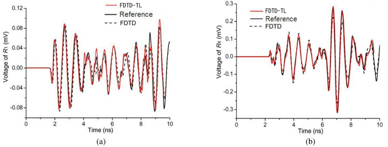
**Figure 4.** Transient terminal voltages for the first example: (a) Transient terminal voltage of  $R_1$  and (b) transient terminal voltage of  $R_4$ .
