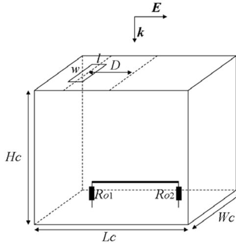
**Figure 5.** Coaxial line in a shielded cavity excited by an incident wave.
