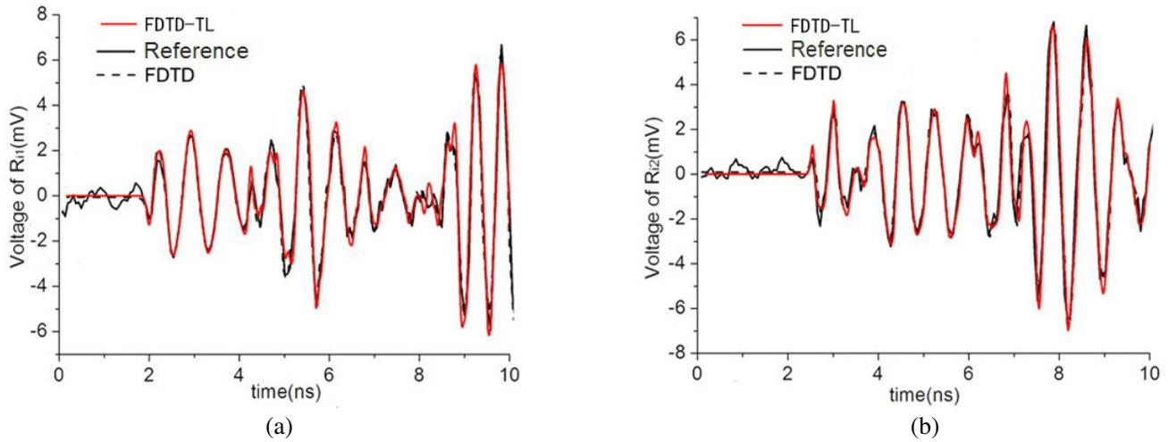
**Figure 6.** Transient voltages of the inner terminal loads: (a) voltage of the load  $R_{i1}$  and (b) voltage of the load  $R_{i2}$ .
