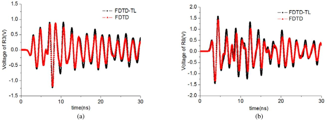
**Figure 8.** Transient voltages of terminal loads: (a) voltage of the load  $R3$  and (b) voltage of the load  $R8$ .
