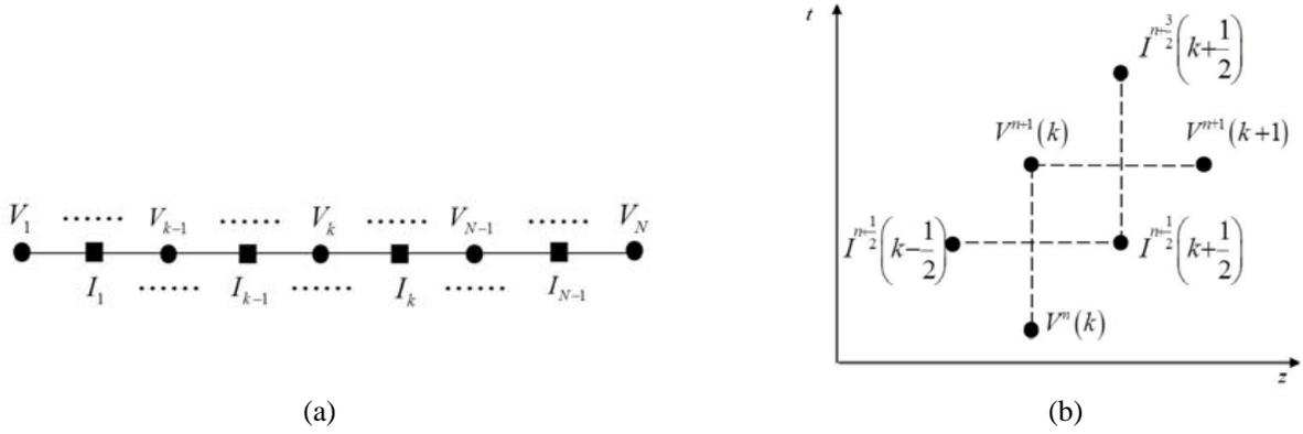
**Figure 2.** Difference scheme of voltage and current: (a) discretization of a line and (b) interlacing of current and voltage nodes in space and time.
