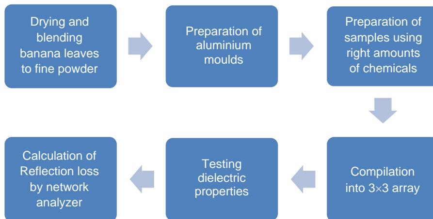
**Figure 2.** Steps for developing and testing microwave absorbers.
