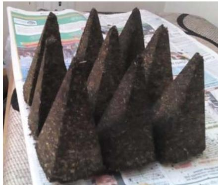
**Figure 4.**  $3 \times 3$  pyramidal microwave absorber.
