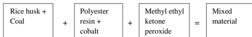
**Figure 3.** The mixing process to make the rice husks pyramidal microwave absorbers.
