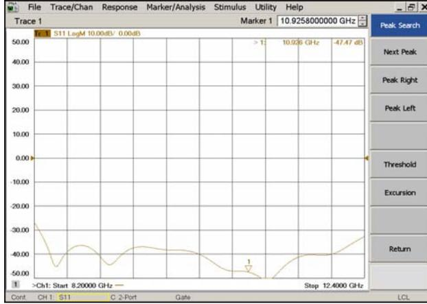
**Figure 8.** Reflection loss performance for  $3 \times 3$  array in the frequency range of 8.2 to 12.4 GHz as shown by VNA.
