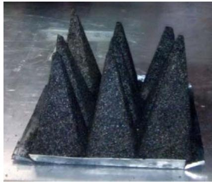
**Figure 5.**  $3 \times 3$  array of microwave pyramidal structure.
