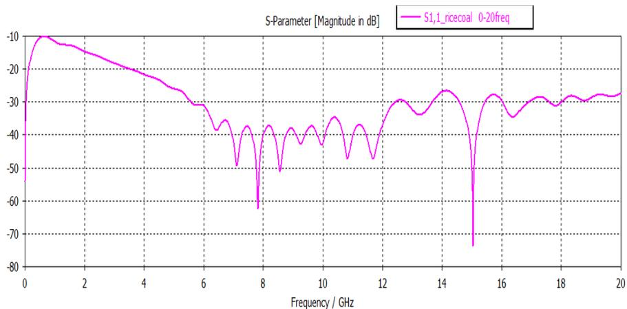
**Figure 11.** Reflection loss performance of ‘rice husk and coal’ in 0 to 20 GHz.
