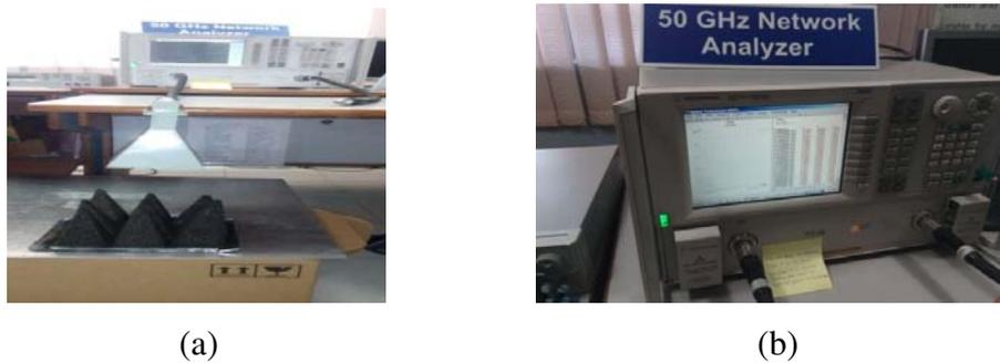
**Figure 7.** (a) Set up for the testing of  $3 \times 3$  pyramidal structure using RCS method. (b) Software set up shown on 50 GHz VNA.
