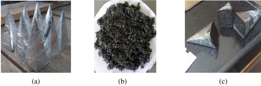
**Figure 4.** (a) Pyramidal moulds. (b) Final mixture. (c) Mixture in the moulds.
