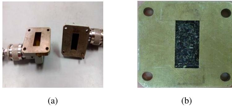
**Figure 6.** (a) WR 90 waveguide and coaxial cables. (b) Material under test.
