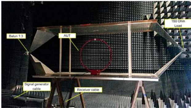
**Figure 10.** Measurement of the reference loop antenna Lindgren 6502.
