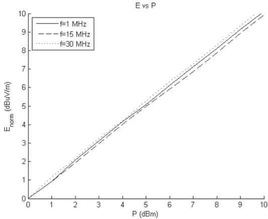
**Figure 5.** Measurement of the linearity of the system.
