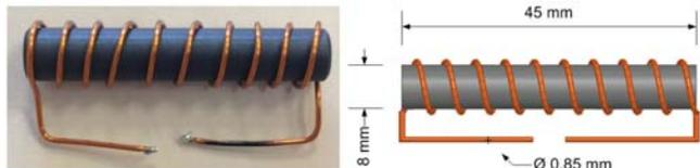
**Figure 14.** Solenoid antenna. Realized and simulated model.
