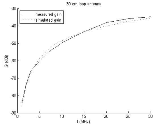
**Figure 13.** Gain measurement of the loop antenna.
