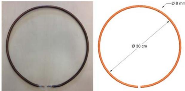
**Figure 12.** Loop antenna. Realized and simulated model.
