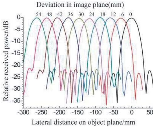
**Figure 12.** Measured beam patterns on the object plane.
