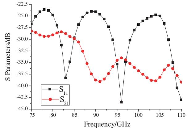
**Figure 5.** Simulation results of coupling between horns.
