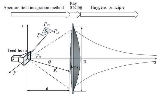
Figure 2. Quasi-optical configuration of the lens antenna.
