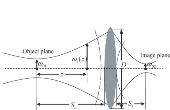
Figure 1. Sketch of Gauss beam transformation.
