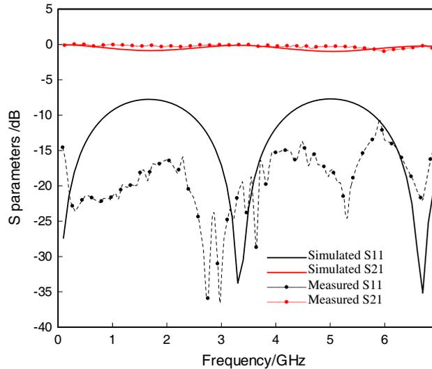
Figure 2. Comparison between simulated and measured  $S$ -parameters.
