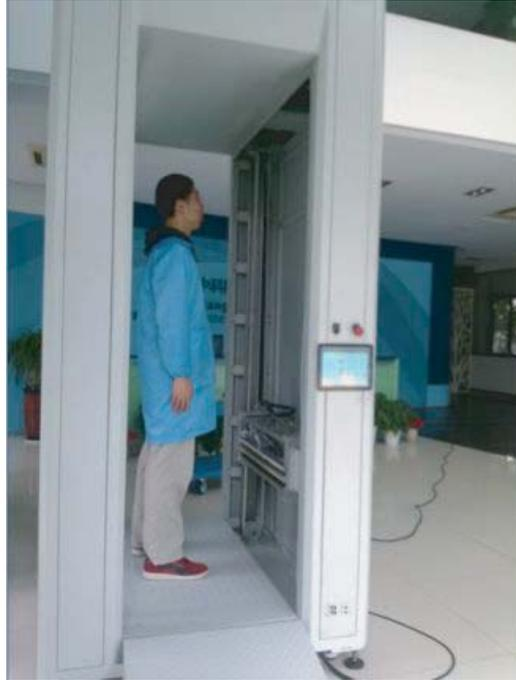
**Figure 3.** The prototype of the wideband mmw imaging system.
