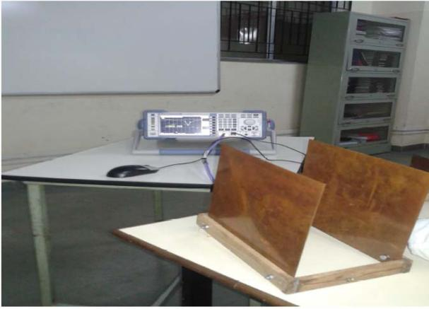
**Figure 5.** Testing setup of the applicator with VNA in the laboratory.
