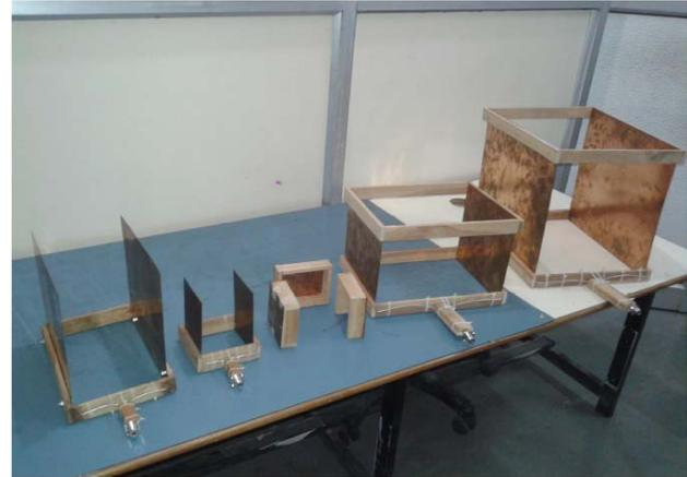
**Figure 6.** Applicators with different distance between plates at 915 MHz & 2450 MHz.
