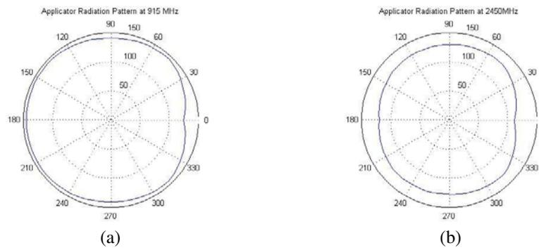
**Figure 9.** The radiation patterns of an applicator at (a) 915 MHz and (b) 2450 MHz.
