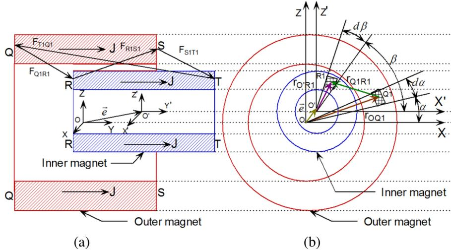
**Figure 2.** (a) Forces acting on inner magnet after a translation  $e$  in  $Y$ - $Z$  plane. (b) Elementary force between two tiny magnetic surfaces on outer and inner magnets in  $Z$ - $X$  plane.
