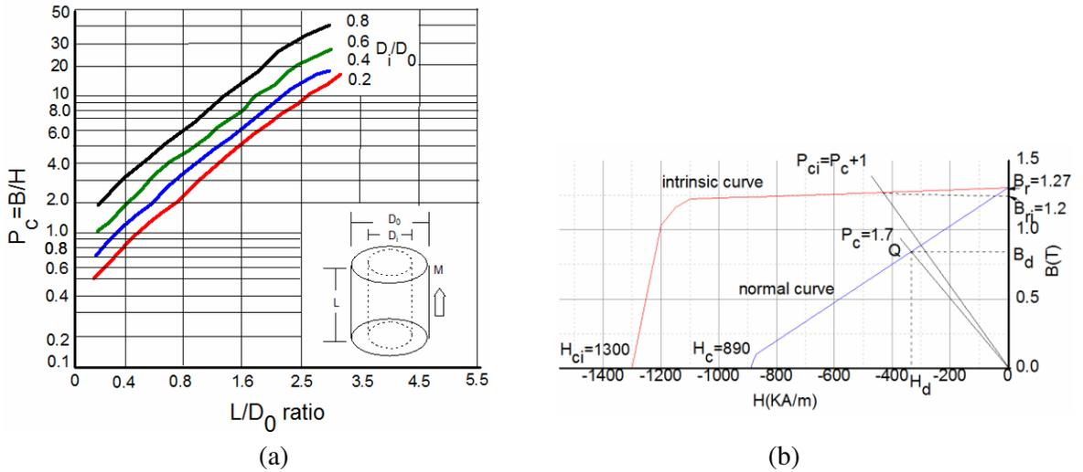
**Figure 3.** (a) Permeance coefficient of ring magnet for different geometries with axial polarization. (b) Calculation of corrected magnetic induction considering self demagnetizing.
