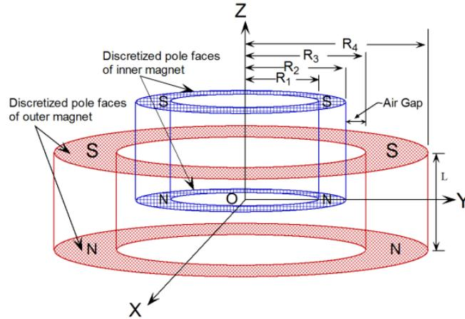
**Figure 1.** Configuration of the passive magnets with dimensions and discretised pole faces.
