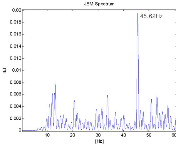
**Figure 6.** The spectrum of input JEM signal.
