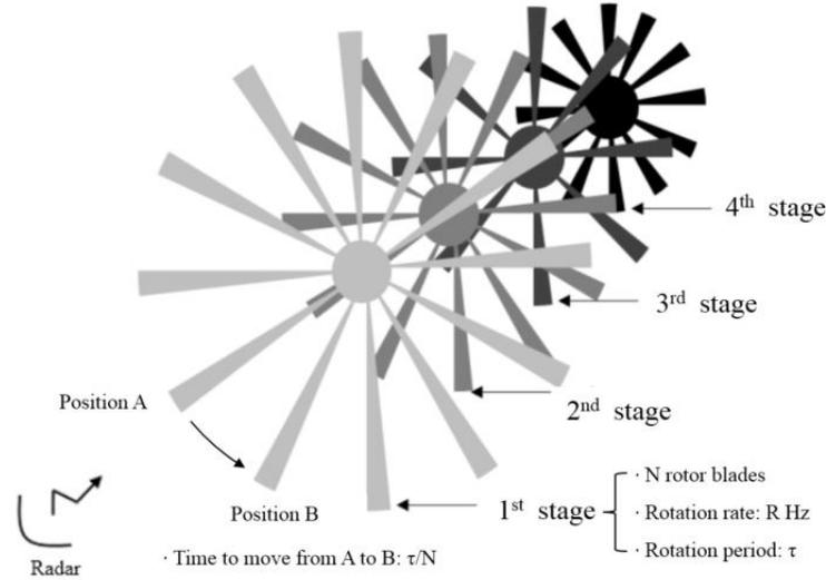
**Figure 1.** Simplified multiple rotor stages and blades of a jet engine.
