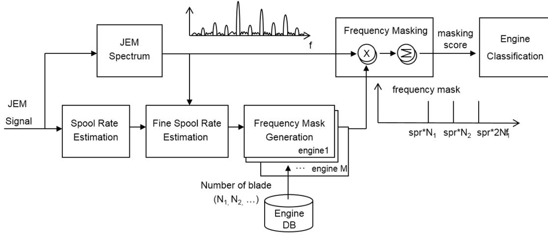
**Figure 4.** Proposed target classification system using frequency mask.
