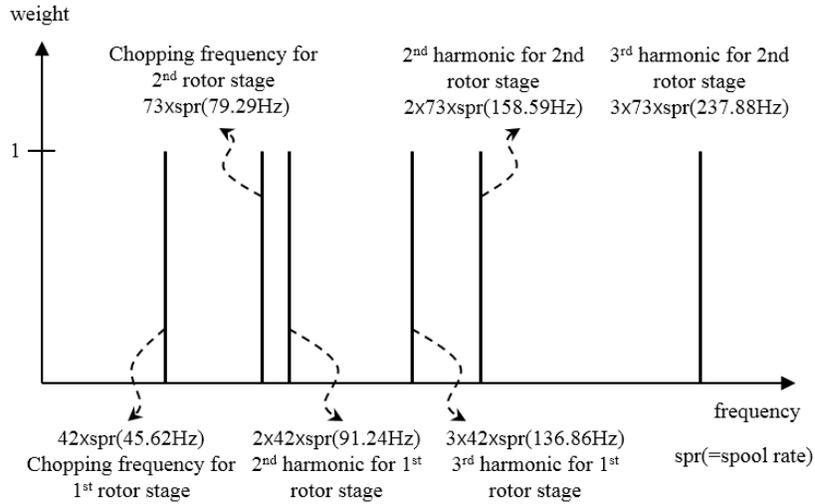
Figure 8. Frequency mask (Blade number of 42 on 1st stage and 73 on 2nd stage).
