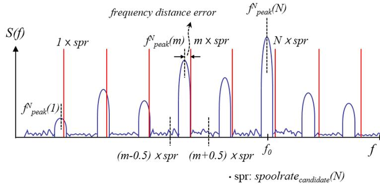
**Figure 5.** Concept of the frequency distance error between the multiples of a spool rate (red solid) and harmonics (blue) in JEM spectrum.
