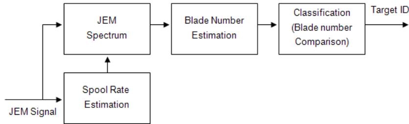
Figure 3. Target classification using JEM signal.
