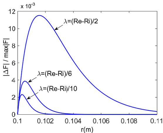
**Figure 3.** The difference between the planar and modified Lorentz forces distributions between the cylinders, for different values of  $\lambda$ .
