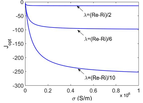
**Figure 6.** The optimal electrical current density as function of the fluid conductivity ( $\Omega i = 1 \text{ Rad/s}$ ,  $B_0 = 1 \text{ T}$ ).
