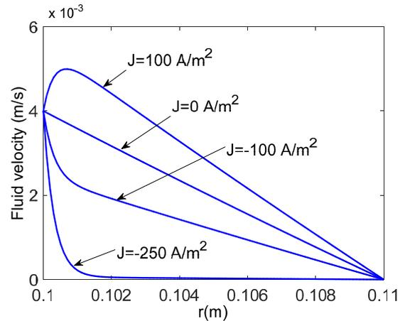
**Figure 4.** Fluid velocity profile between the cylinders for different values of the applied current ( $\sigma = 5 \text{ S/m}$ ,  $\lambda = [R_e - R_i]/10$ ).
