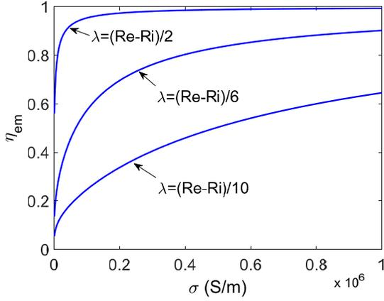
**Figure 5.** The control efficiency as function of the fluid conductivity for different values of  $\lambda$  ( $J = -100 \text{ A/m}^2$ ).
