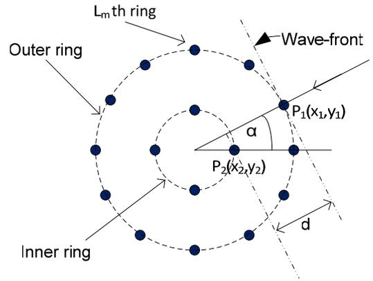
**Figure 2.** Geometry of concentric circular antenna array system.
