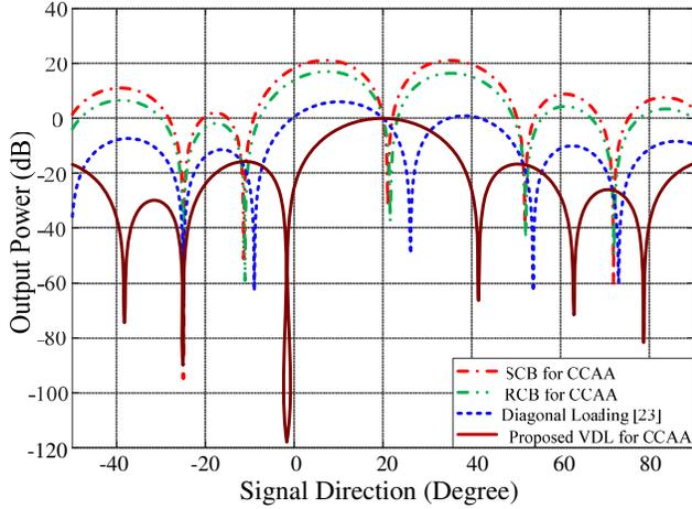
**Figure 5.** Comparison of the Power pattern of SCB, RCB, Diagonal loading method [23] and proposed VDL method for CCAA beamformer with  $1^\circ$  look direction error (assume signal direction =  $20^\circ$  and actual signal direction =  $21^\circ$ ) and in the presence of an interfering signal at  $-25^\circ$ .
