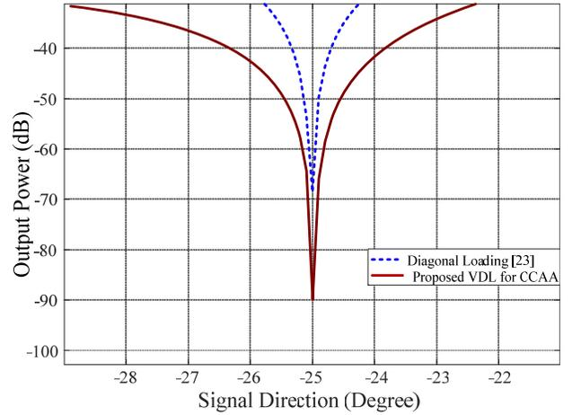
**Figure 6.** Comparison of the interference cancellation capability CCAA based beamformer with Diagonal Loading Technique [23] and proposed VDL technique.
