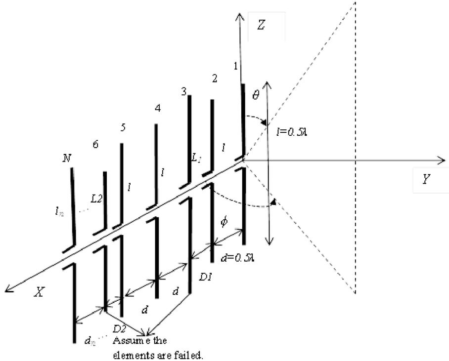
**Figure 1.** Geometry of a linear array with failed and non-defective element.
