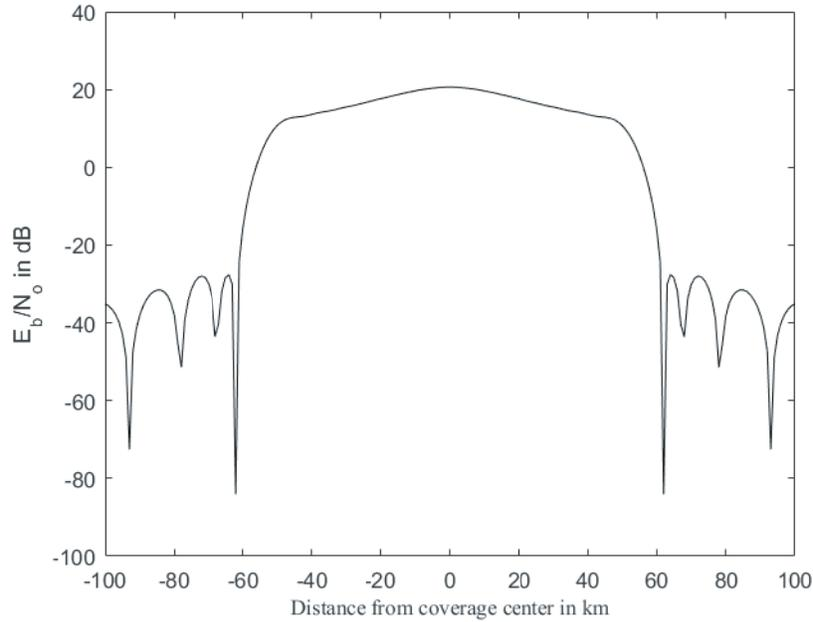
**Figure 11.** Profile view of the HAP  $\frac{E_b}{N_o}$  in dB.
