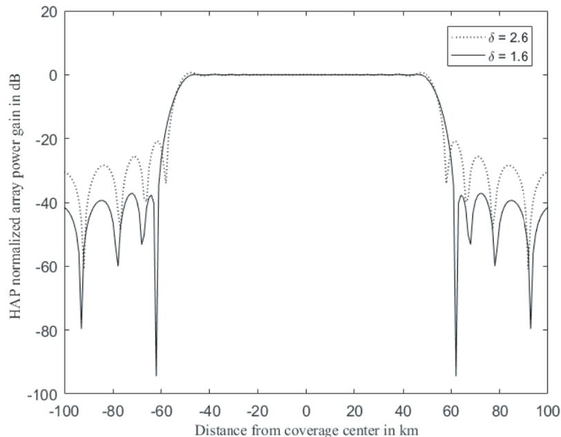
**Figure 17.** Effect of the smoothing function on the normalized array power gain.
