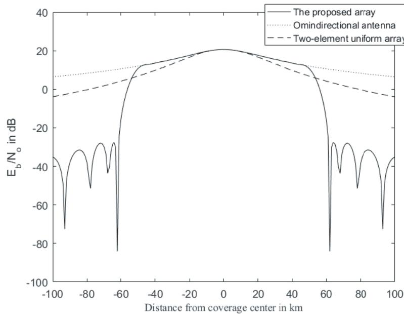
Figure 14.  $\frac{E_b}{N_o}$  profile for three antenna systems for aerial coverage from HAP.
