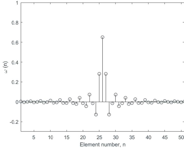
**Figure 7.** Weighting function profile for 100 km diameter coverage for HAP at 20 km high.
