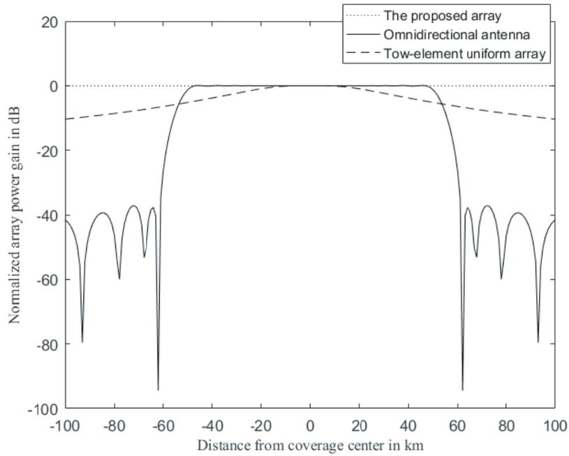
Figure 13. Normalized antenna power gain of three antenna systems for aerial coverage from HAP.
