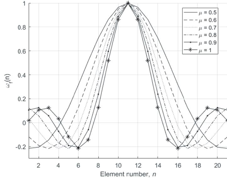
**Figure 3.** Flattening function profile at different beamwidth control factor ( $\mu$ ).
