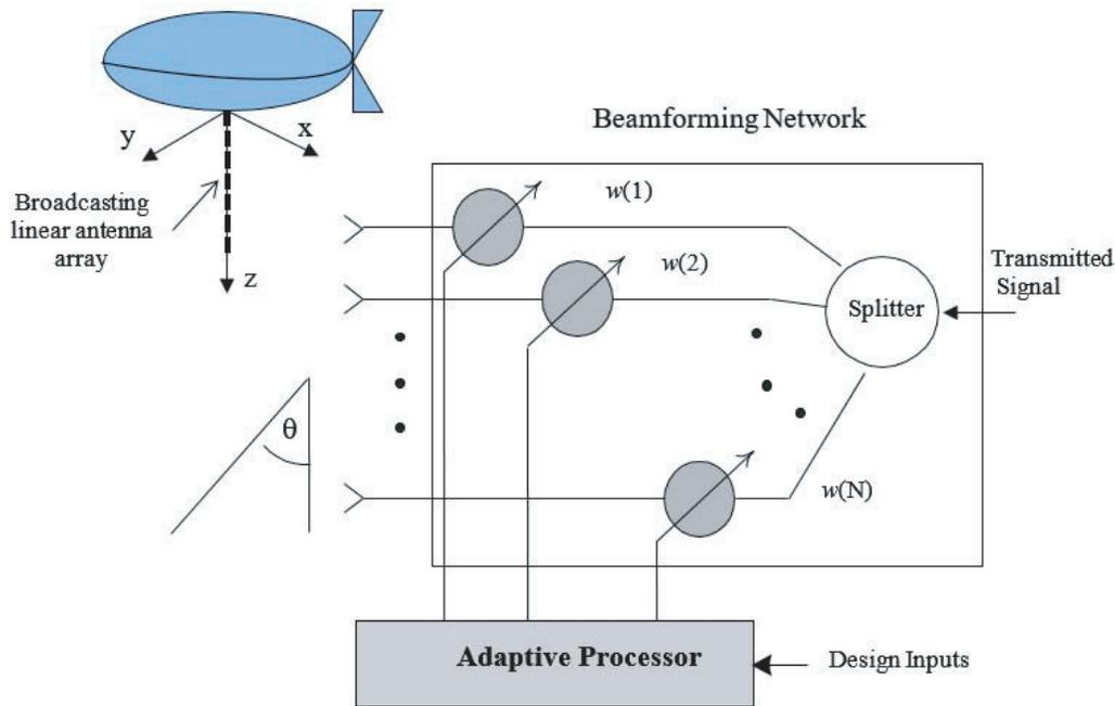
**Figure 2.** Beamforming system for the vertical broadcasting array onboard AP.
