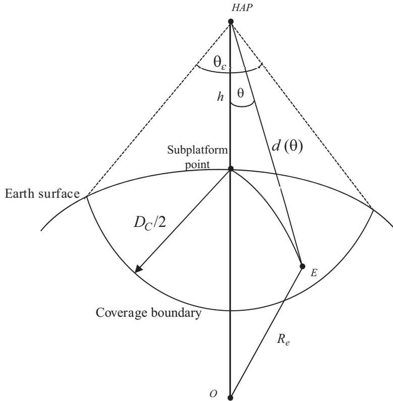
**Figure 6.** Geometry of HAP broadcasting system for slant range calculation.
