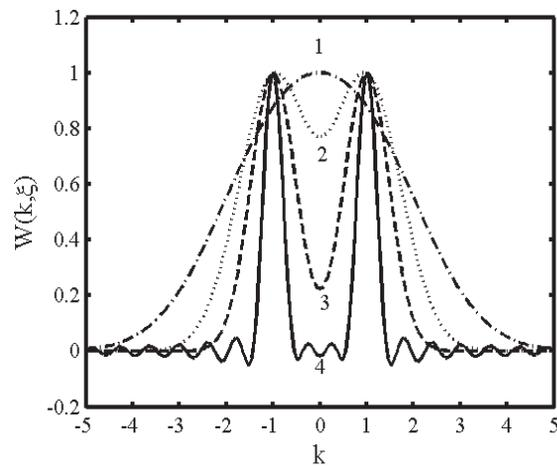
**Figure 5.** Spatial power spectrum of a scattered field.
