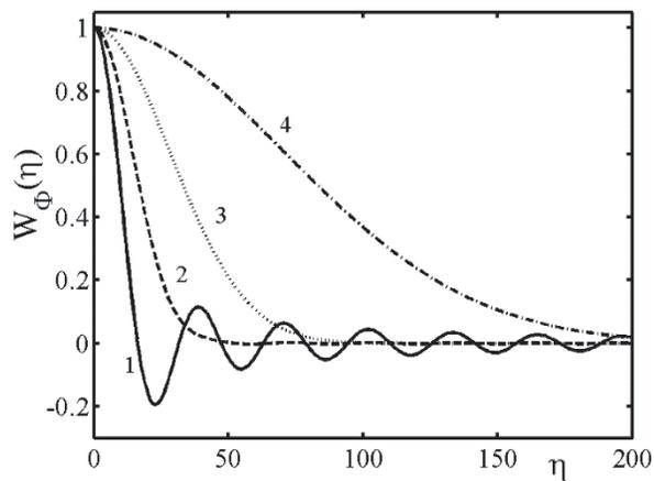
**Figure 3.** Correlation function as a function of distance between observation points in the principle plane for different characteristic special scale of plasma irregularities  $l_{||}$ .
