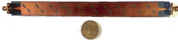
**Figure 7.** Fabricated prototype of asymmetrical LWA.
