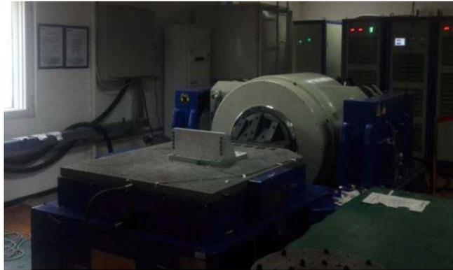
Figure 7. Electrical shaking table.
