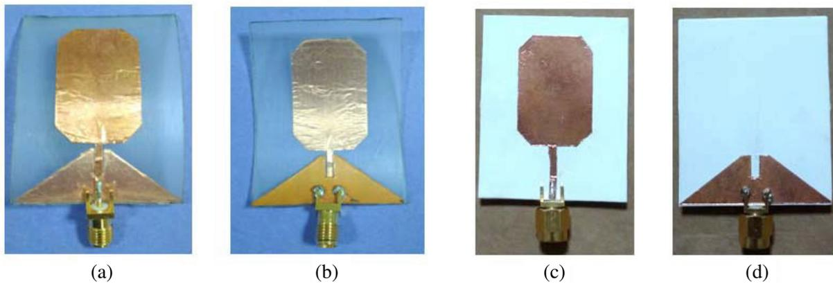
**Figure 2.** Front and rear views of fabricated antennas, (i) polyamide antenna, (a) front view, (b) rear view, (ii) Teslin paper antenna, (c) front view, (d) rear view.
