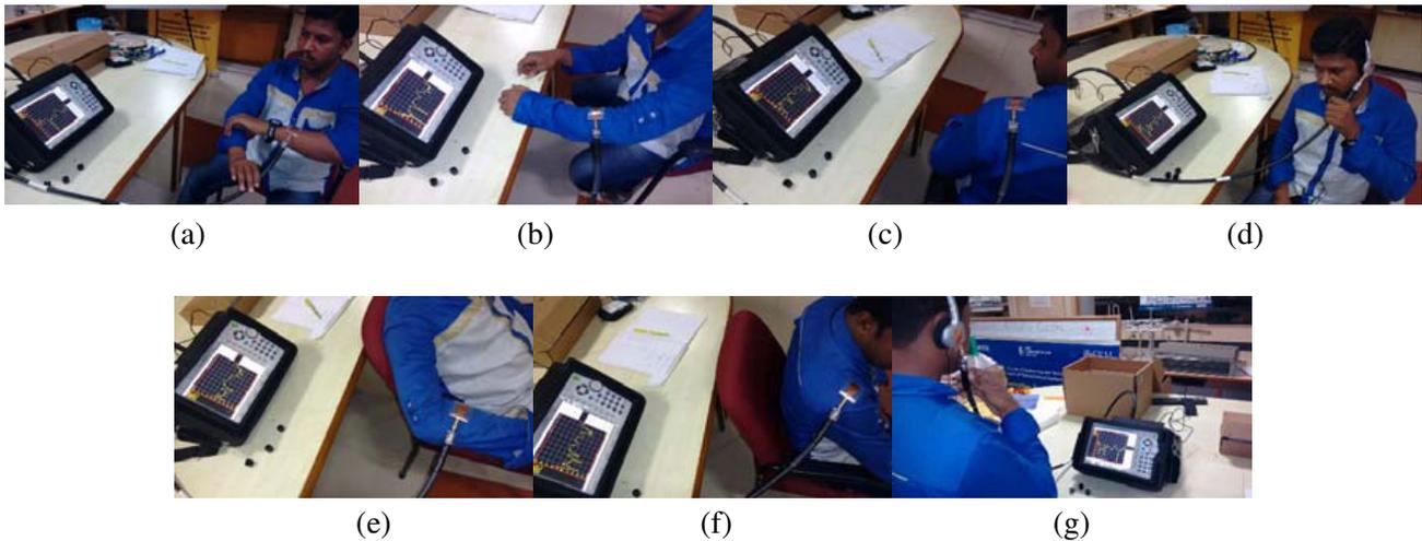
**Figure 5.** Measurement setup for Antenna placed in different locations, (i) on left-side, (a) wrist, (b) hand, (c) shoulder, (d) head phone, (ii) on the right-side of the body, (e) hand, (f) shoulder, (g) head phone.
