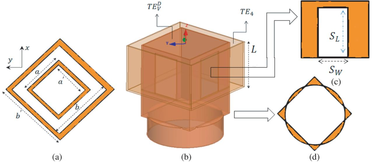
**Figure 1.** (a) Aperture:  $\{a', a, b, b'\} = \{26, 29, 35, 43\}$  mm. (b) Proposed matched feed structure:  $L = 22$  mm. (c) Slot:  $\{S_L, S_W\} = \{20, 12\}$  mm. (d) Junction between standard circular waveguide (diameter 32.512 mm) and diagonal waveguide.
