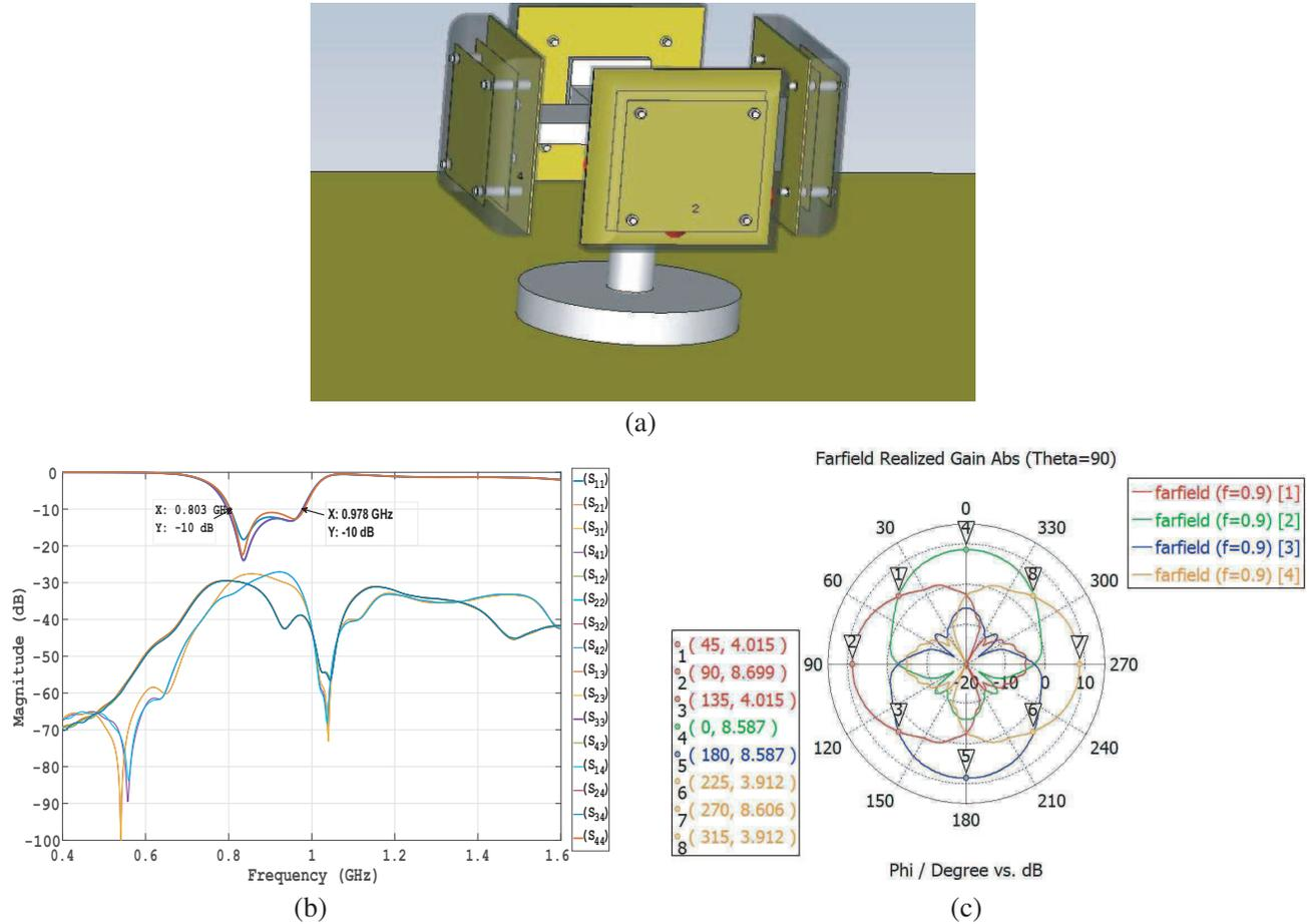
**Figure 3.** (a) Beam switchable antenna structure. (b) Simulated  $S_{11}$ -parameter for beam switchable antenna on the vehicle rooftop of size 1700 mm  $\times$  1100 mm. (c) Azimuth plane patterns for four-element antenna.
