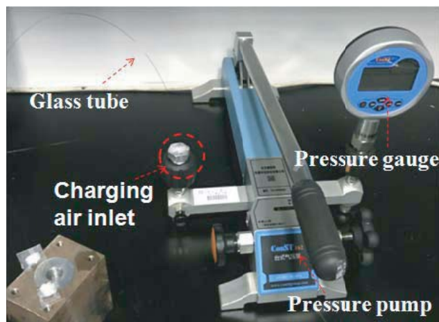
Figure 2. Experimental setup of pressure filling system.
