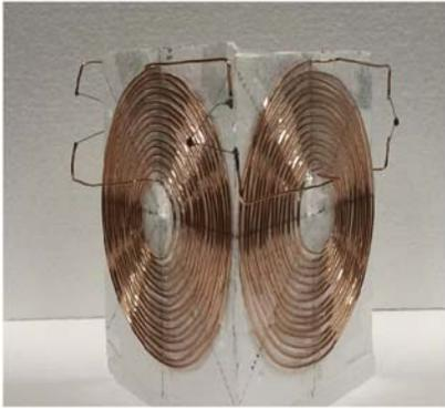
**Figure 7.** A prototype of the 3D spiral resonator.
