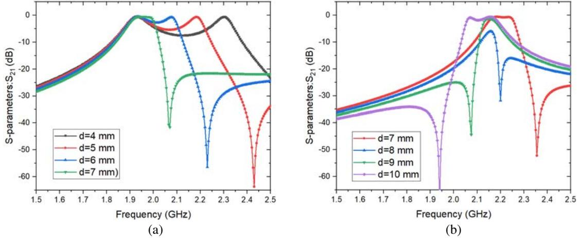
**Figure 3.** Simulated response of transmission zero located at (a) upper side band of the center frequency of 1.95 GHz (b) lower side band of the center frequency of 2.14 GHz with different length of loaded stepped-impedance.
