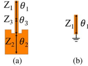
**Figure 2.** (a) Even-mode resonator (b) Odd-mode resonator.
