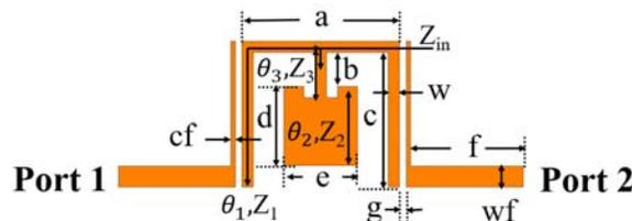
**Figure 1.** Schematic diagram of dual-mode microstrip stepped-impedance resonator.
