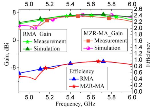
**Figure 8.** Gains and efficiencies of the RMA and the MZR-MA.
