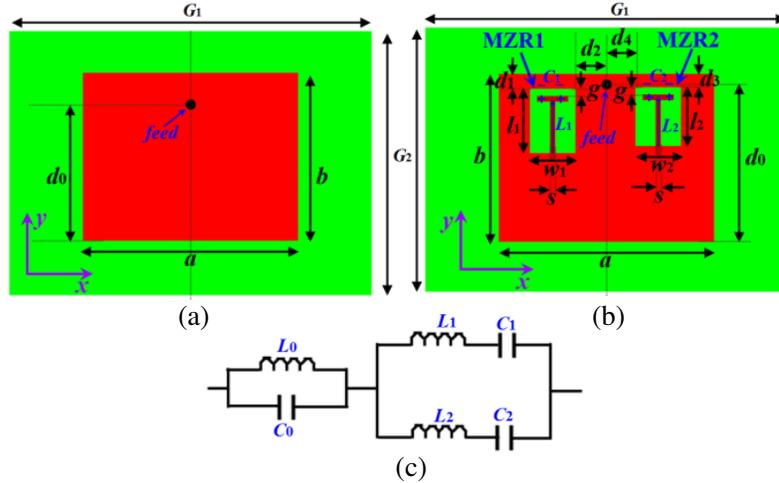
**Figure 1.** Schematic view of the antennas. (a) The RMA, (b) the proposed MZR-MA, and (c) equivalent circuit model of the proposed MZR-MA.
