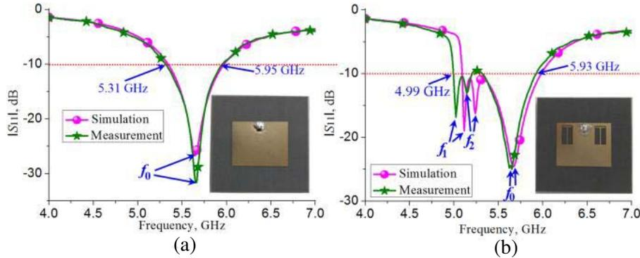
**Figure 4.** Simulated and measured  $|S_{11}|$  of the antennas. (a) RMA, and (b) MZR-MA.
