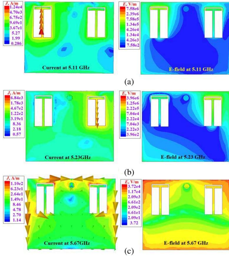
**Figure 5.** Current/ $E$ -field distributions of the MZR-MA. (a)  $f_1 = 5.11$  GHz, (b)  $f_2 = 5.23$  GHz, and (c)  $f_0 = 5.67$  GHz.
