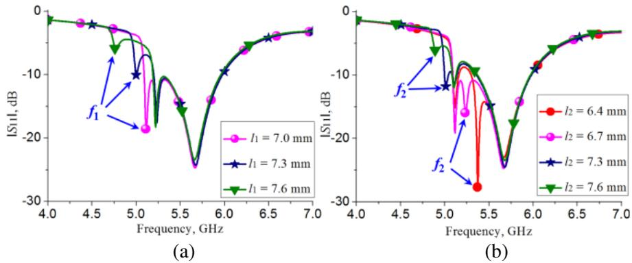
**Figure 6.** Parametric study. (a)  $l_1$ , and (b)  $l_2$ .
