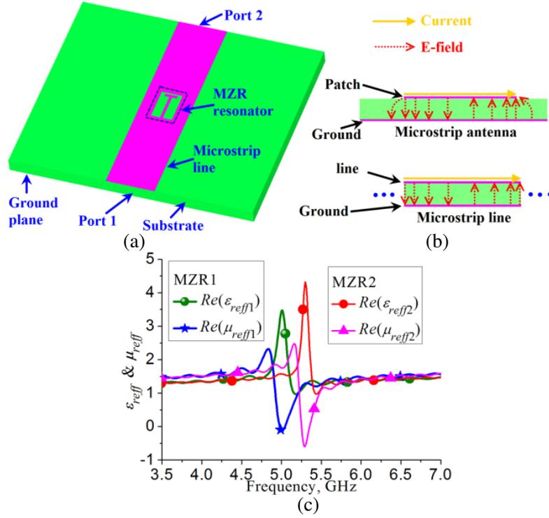
**Figure 2.** The constitutive parameters of the MZR resonators. (a) Simulation model, (b) currents and  $E$ -fields of the microstrip antenna and microstrip line, and (c) results.
