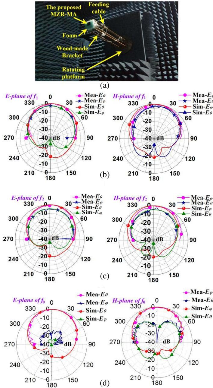
**Figure 7.** Radiation patterns. (a) The measuring environment, (b)  $f_1$ , (c)  $f_2$ , and (d)  $f_0$ .
