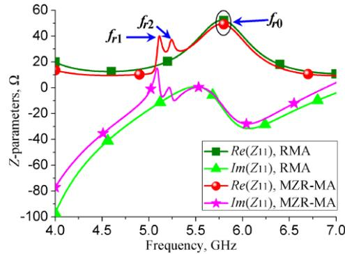
**Figure 3.**  $Z$ -parameters of the RMA and MZR-MA.
