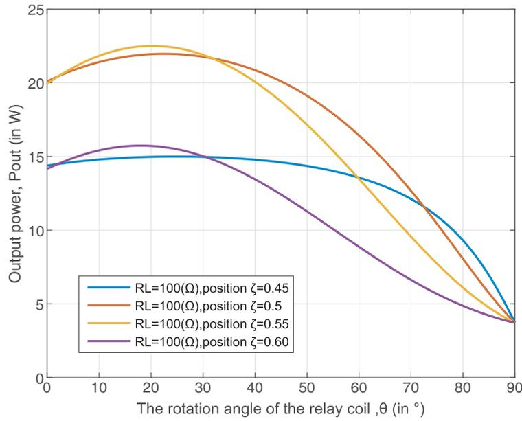
**Figure 5.** Relationship between output power  $P_{out}$  and rotation angle  $\theta$  of relay coil, when load  $R_L = 100 \Omega$ .
