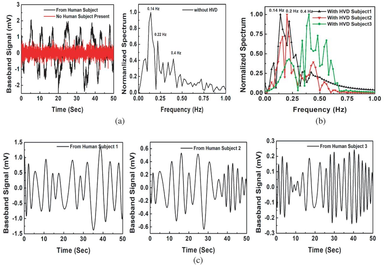
**Figure 6.** When three human subject are present — all breathing at different rates, (a) respiration signal without HVD and its normalized spectrum, (b) normalized spectrum of extracted respiration signals with HVD algorithm and (c) extracted respiration signals with HVD algorithm.
