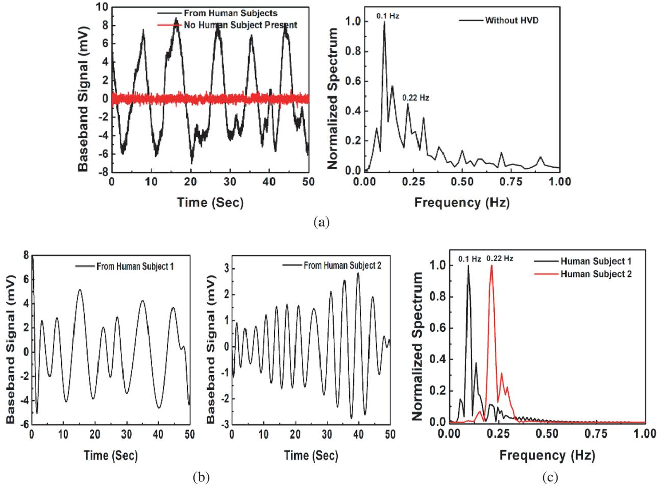
**Figure 5.** When two human subject are present one normal breathing and other slow breathing, (a) respiration signal without HVD and its normalized spectrum, (b) extracted respiration signals with HVD algorithm and (c) normalized spectrum of extracted respiration signals.
