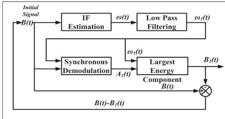
Figure 2. Block diagram of Hilbert vibrational decomposition (HVD).
