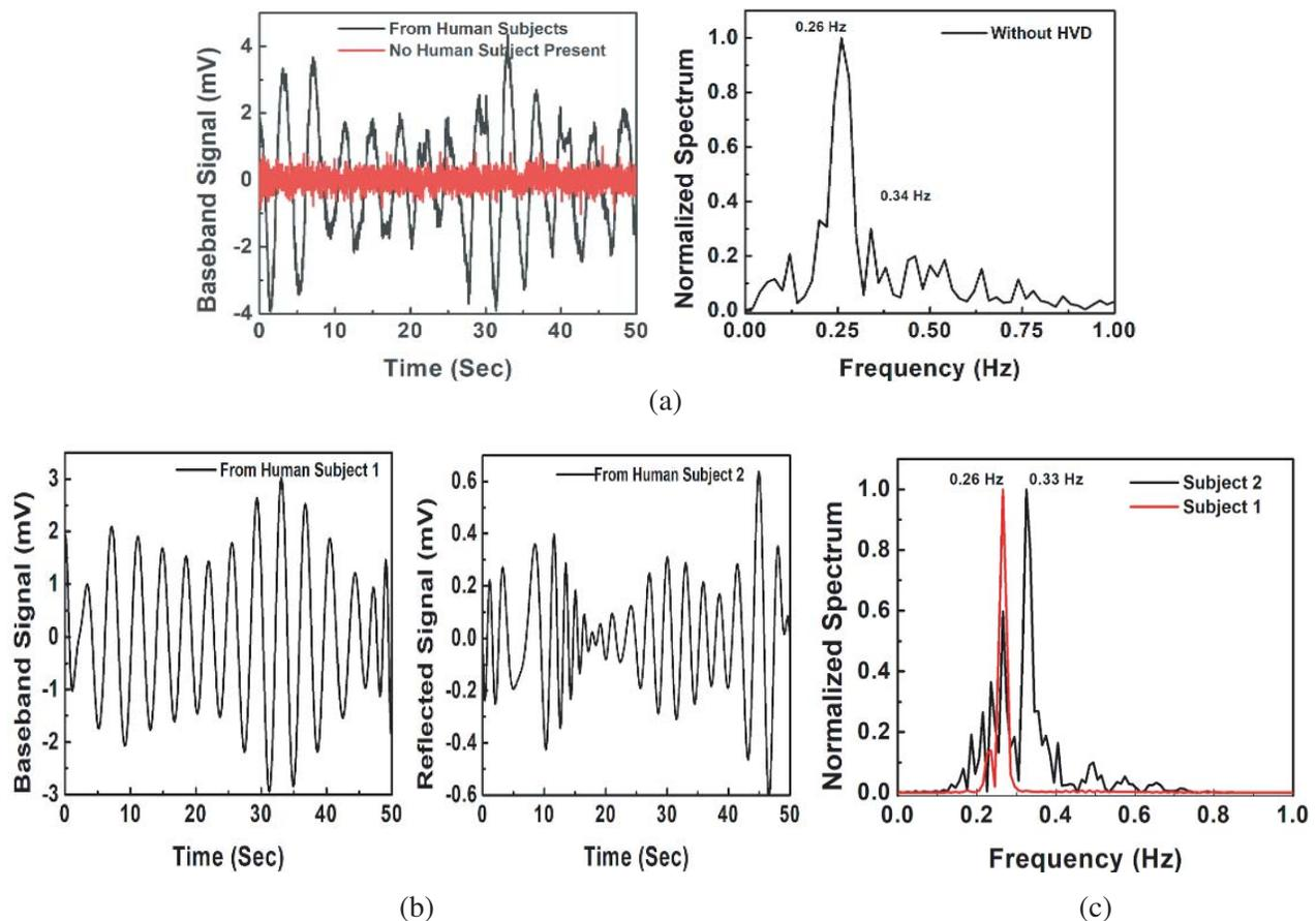
**Figure 4.** When both human subjects are breathing normal, (a) respiration signal without HVD and its normalized spectrum, (b) extracted respiration signals with HVD and (c) normalized spectrum of extracted respiration signals.
