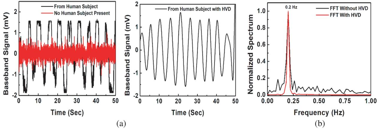
**Figure 7.** When antennas are 2 meter away from the initial position and human subject is breathing normal, (a) respiration signal without HVD and with HVD algorithm and (b) normalized spectrum of respiration signal.
