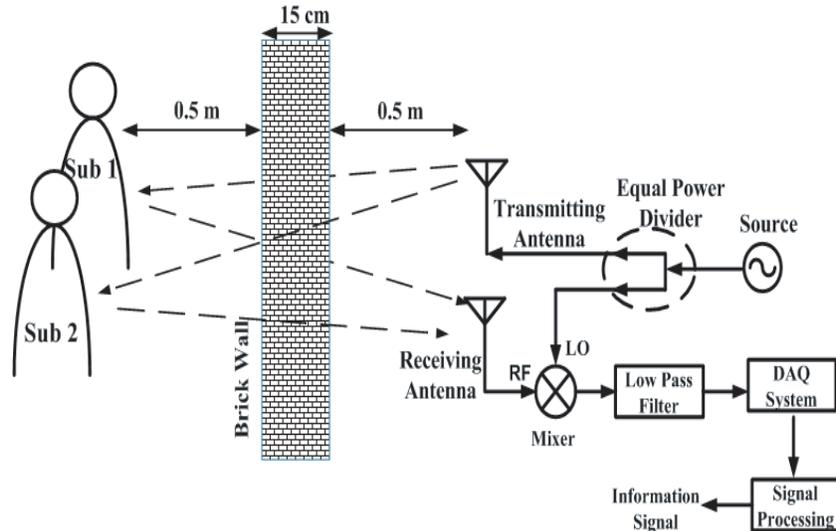
**Figure 1.** Block diagram of direct demodulation system.
