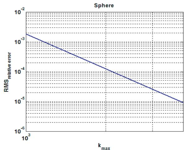
Figure 10. RMSRE versus  $K_{\max}$  for the PEC sphere.
