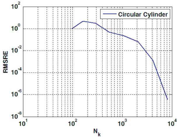
Figure 7. RMSRE versus  $N_k$  for circular cylinder.
