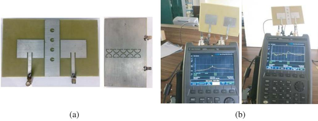
**Figure 13.** (a) Fabricated antenna front and back view. (b) Measurement setup of VNA (with & without CSRR & circle slots).
