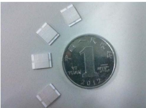
**Figure 11.** Actual processed passband filter.
