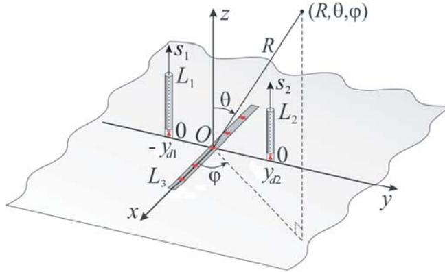
**Figure 1.** The geometry of the Clavin vibrator-slot radiator.
