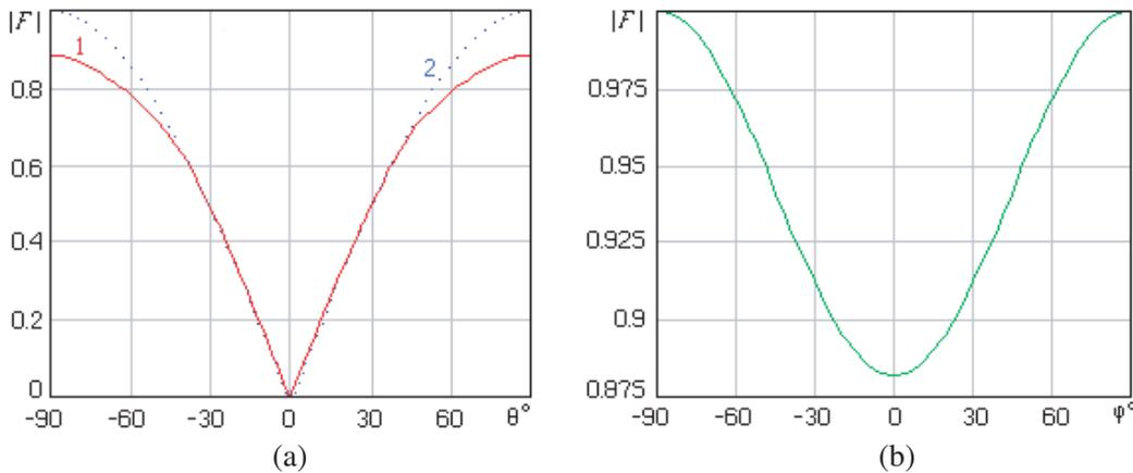
**Figure 5.** The RPs of two active monopoles with parameters  $L_v = 0.284\lambda_a$  and  $y_v = 0.078\lambda_a$  at the alternative frequency: (a) 1 — in  $E$ -plane ( $\varphi = \pi/2$ ), 2 — in  $H$ -plane ( $\varphi = 0$ ); (b) in plane  $\theta = \pm 90^\circ$ .
