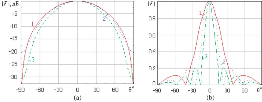
**Figure 4.** The RPs of radiating structures at the main frequency: (a) single Clavin element: 1 — in  $H$ -plane with parameters  $L_v = 0.3125\lambda$ ,  $y_v = 0.086\lambda$ ; 2 — in  $E$ -plane with parameters  $L_v = 0.3125\lambda$ ,  $y_v = 0.086\lambda$ , 3 — in  $E$ -plane with parameters  $L_v = 0.3\lambda$ ,  $y_v = 0.086\lambda$ ; (b) array of Clavin elements: 1 —  $N_x = N_y = 3$ , 2 —  $N_x = N_y = 5$ , 3 —  $N_x = N_y = 7$ .
