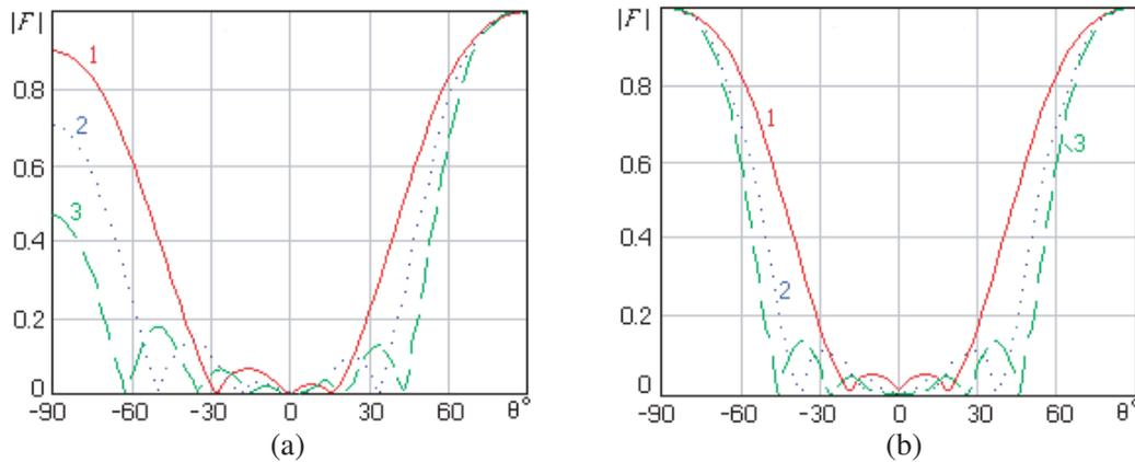
**Figure 6.** RPs of the antenna arrays with different number of radiators at the alternative frequency: 1 —  $N_x = N_y = 3$ , 2 —  $N_x = N_y = 5$ , 3 —  $N_x = N_y = 7$ . (a) Without phase compensation; (b) with phase compensation.
