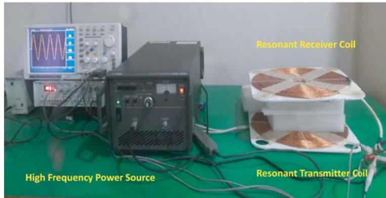
**Figure 3.** Practical demonstration of MRC based WPT System.
